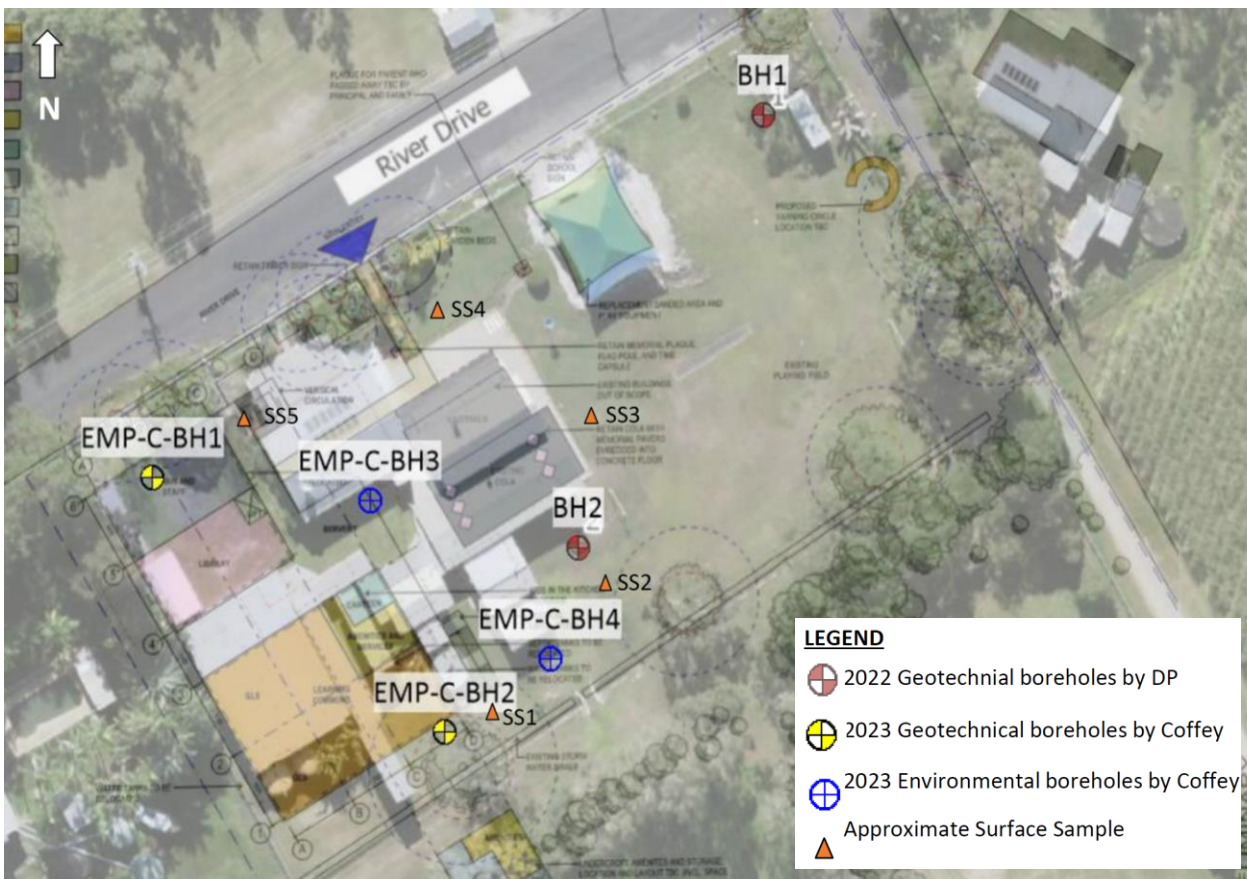
Figure 13 Borehole and sampling locations Empire Vale (Source: Tetra Tech Coffey)
