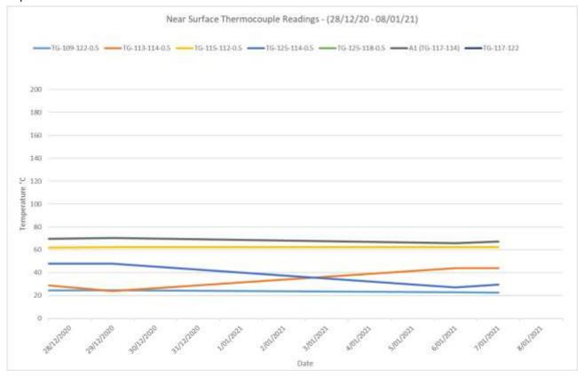
The near-surface temperature appears to fluctuate seasonally across the surface of the northwest hotspot grid monitoring area.
