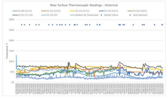
The near-surface temperature appears to fluctuate seasonally across the surface of the northwest hotspot grid monitoring area.
