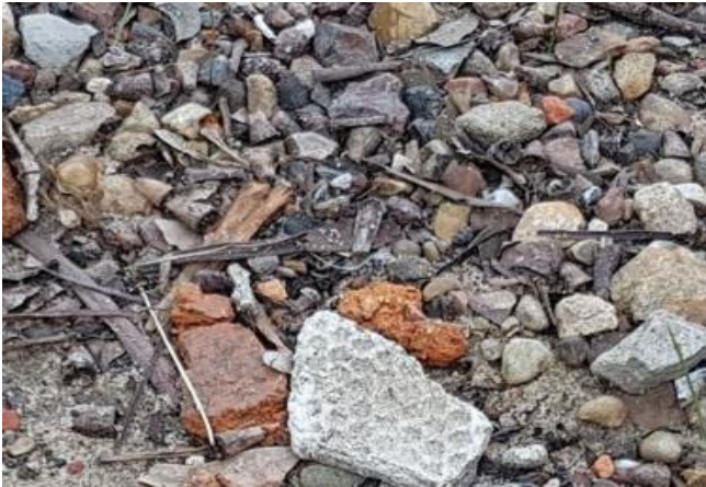
Asbestos Cement (AC) Fragments/Debris such as fibro are often present in or on the soil surface as a result of incomplete clean-up following the past-demolition of structures that contained asbestos and the widespread presence of asbestos-containing fill. The debris can also be found in recycled aggregate.
