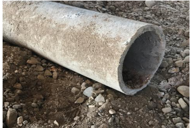
Asbestos Cement (AC) piping , asbestos cement water and sewer pipes.
