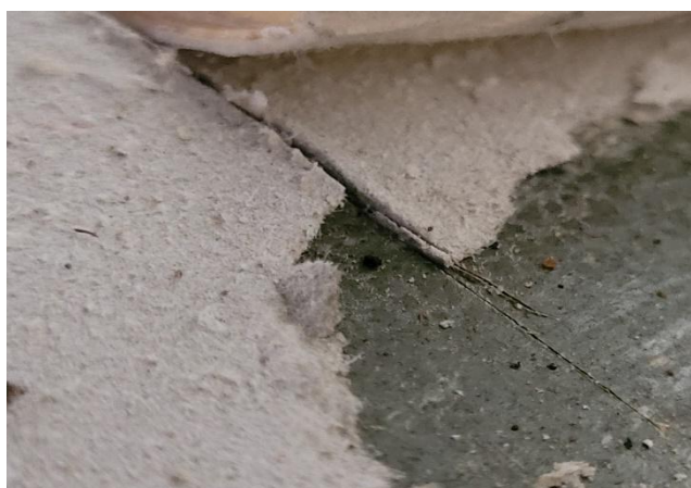
Asbestos-backing paper , can be used to line to underside of vinyl flooring.
