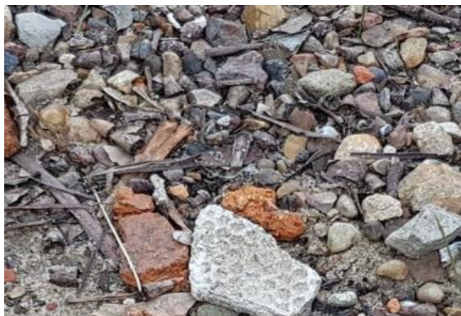
Asbestos Cement (AC) Fragments/Debris such as fibro are often present in or on the soil surface as a result of incomplete clean-up following the past-demolition of structures that contained asbestos and the widespread presence of asbestos-containing fill. The debris can also be found in recycled aggregate.
