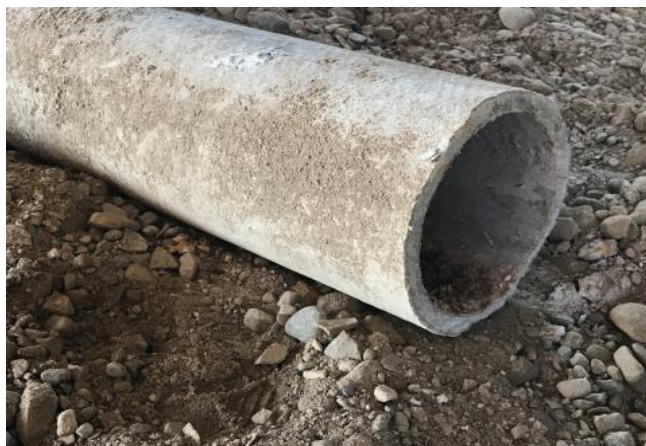
Asbestos Cement (AC) piping , asbestos cement water and sewer pipes.
