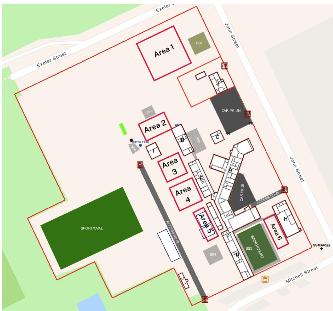
Excavation of existing soil and mulch will take place in areas 1 and 5 with geofabric installed to limit the possibility of further asbestos being found at ground level. Areas 2, 3, 4 and 6 will have geofabric laid before being covered by new turf, mulch and soil.
