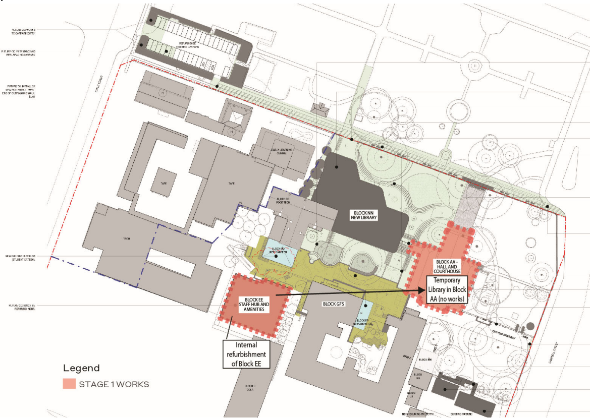
Figure 1 Extent of Stage 1 Works – Internal Refurbishment of Block EE
