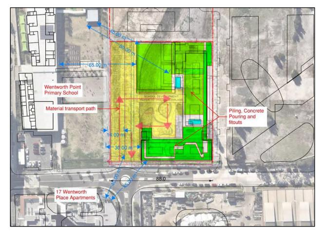
**Figure 3. Noise Sensitive Receiver Locations and Distances**
