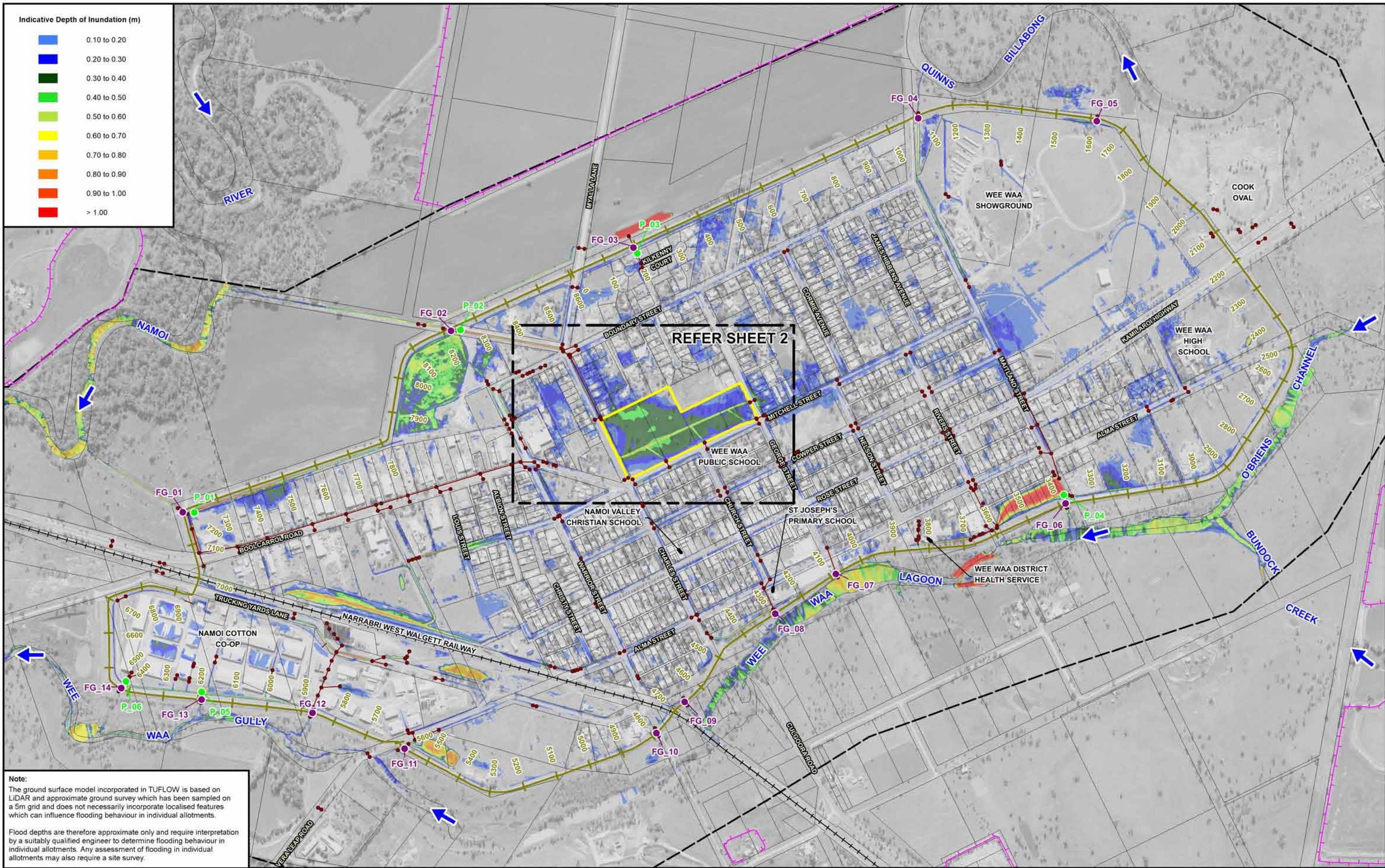
INDICATIVE EXTENT AND DEPTH OF INUNDATION INTERNAL TO TOWN LEVEE PRE-REF AND SSD CONDITIONS - 20% AEP Figure 4 (Sheet 1 of 2)
