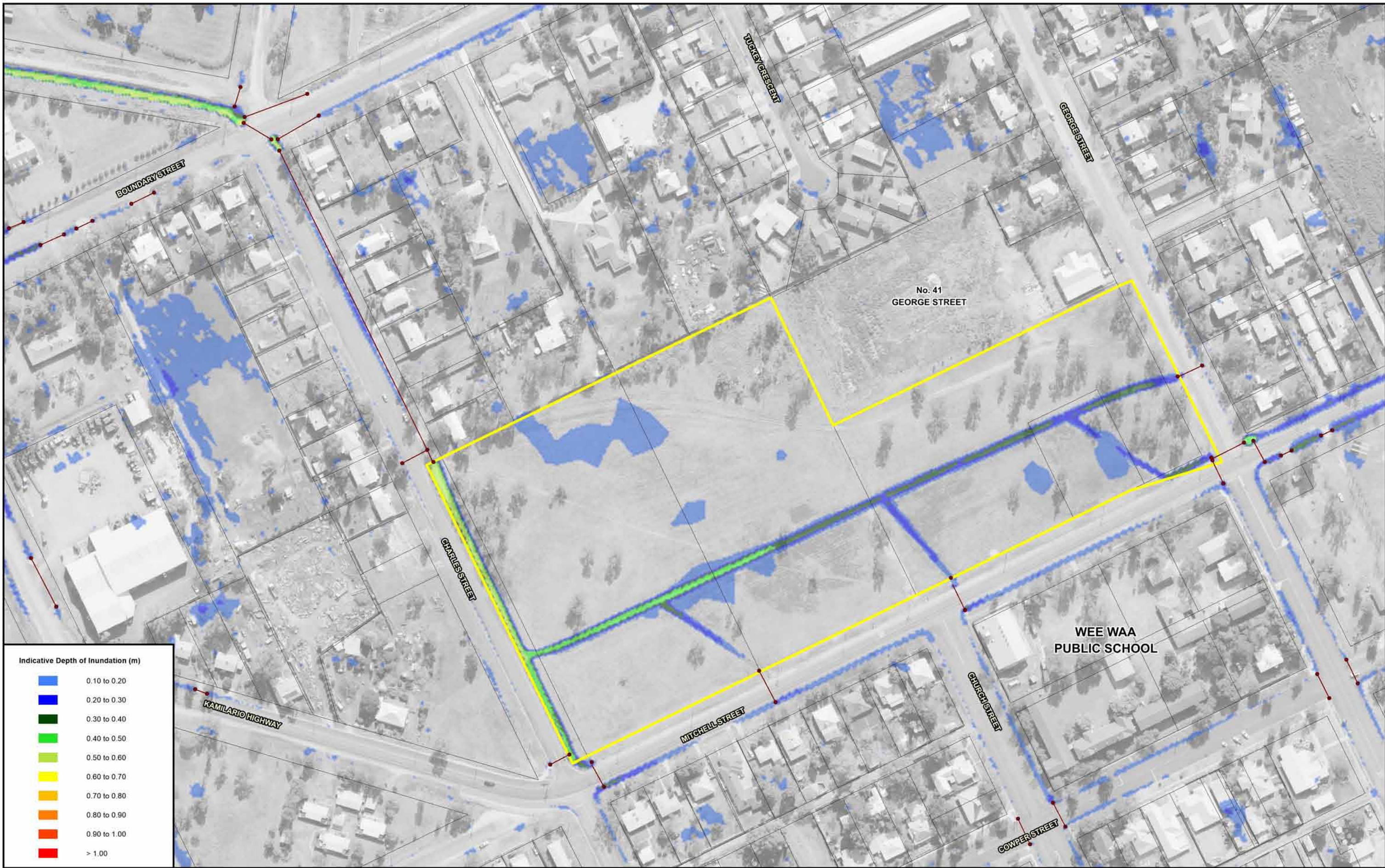
INDICATIVE EXTENT AND DEPTH OF INUNDATION INTERNAL TO TOWN LEVEL PRE-REF AND SSD CONDITIONS - 1 EY
