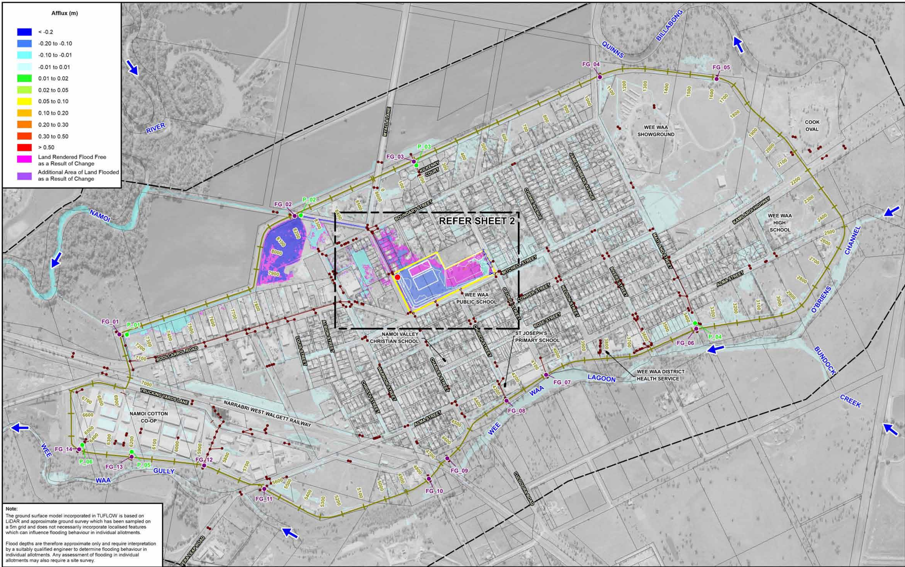
Figure 12 (Sheet 1 of 2) IMPACT OF STAGE 2 SSD WORKS ON FLOOD BEHAVIOUR INTERNAL TO TOWN LEVEL 20% AEP
