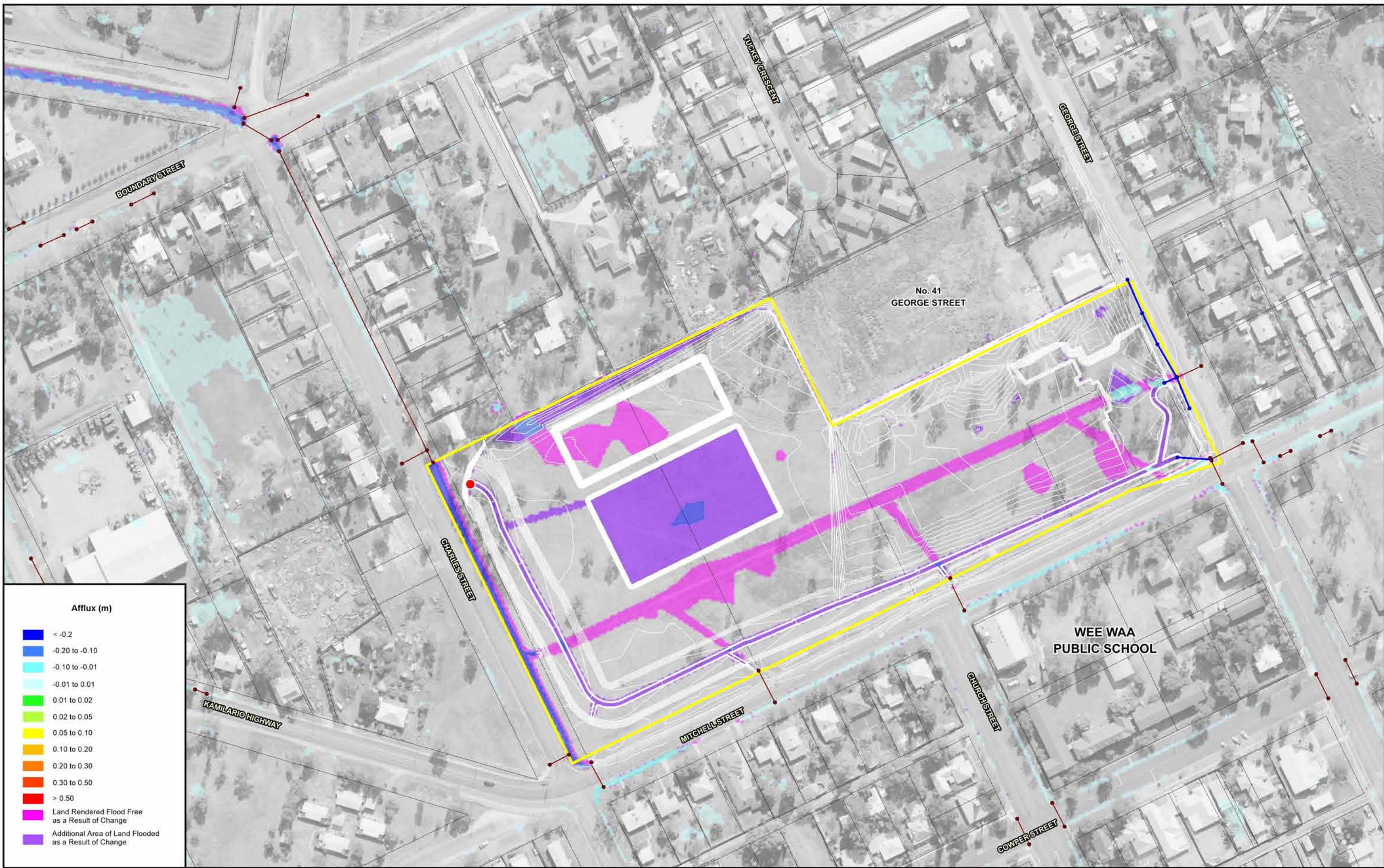
Figure 11 (Sheet 2 of 2) IMPACT OF STAGE 2 SSD WORKS ON FLOOD BEHAVIOUR INTERNAL TO TOWN LEVEL 1 EY
