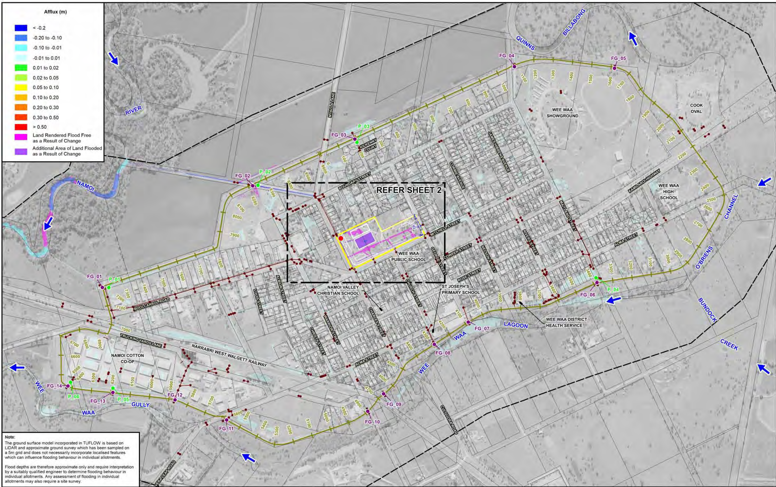
Figure 11 (Sheet 1 of 2) IMPACT OF STAGE 2 SSD WORKS ON FLOOD BEHAVIOUR INTERNAL TO TOWN LEVEL 1 EY
