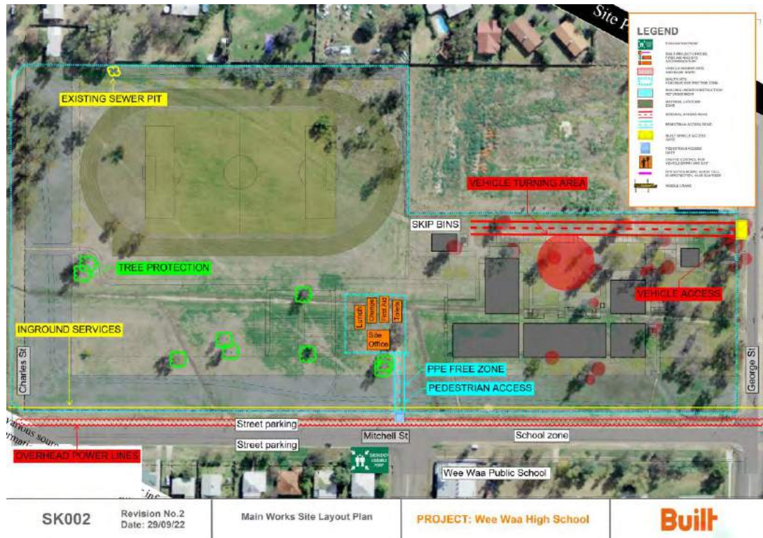
FIGURE 4 - SKIP BIN PICK UP LOCATION
