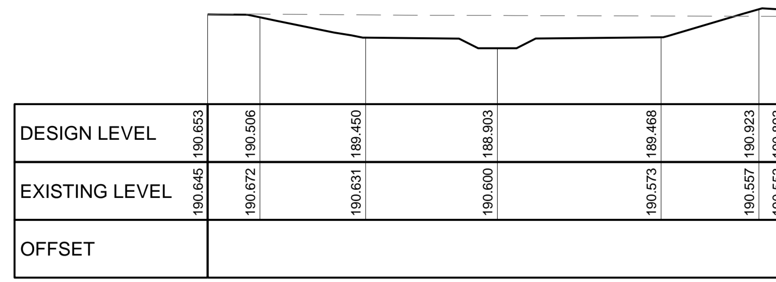
CHAINAGE 500.00 HORIZONTAL SCALE 1:200 VERTICAL SCALE 1:200
