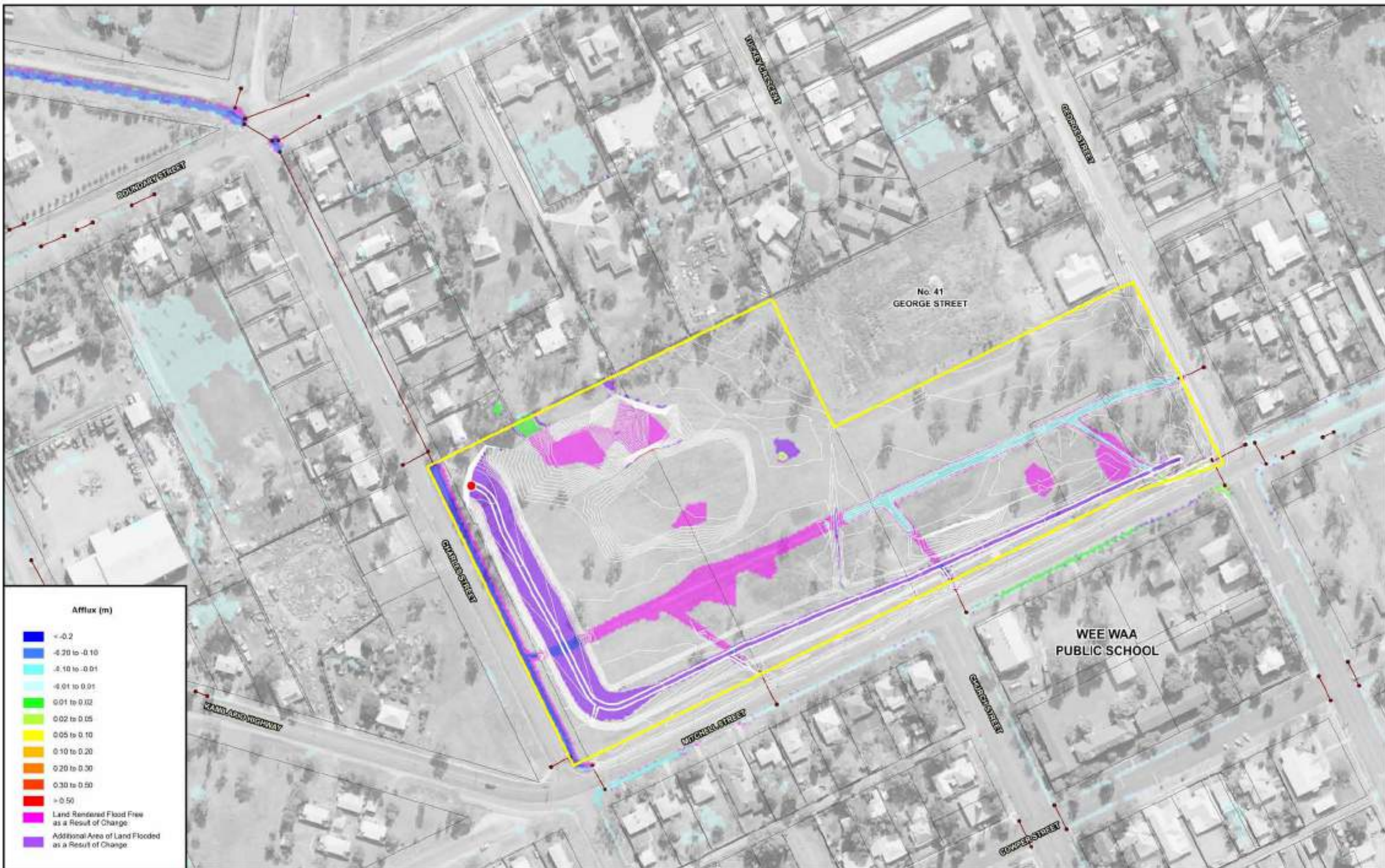
IMPACT OF STAGE 1 SSD WORKS ON FLOOD BEHAVIOUR INTERNAL TO TOWN LEVELLE 1 EY Figure 7 (Sheet 2 of 2)
