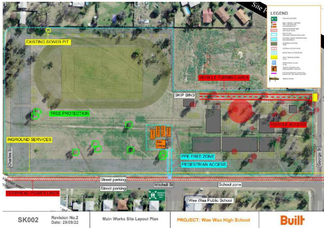
FIGURE 4 - SKIP BIN PICK UP LOCATION
