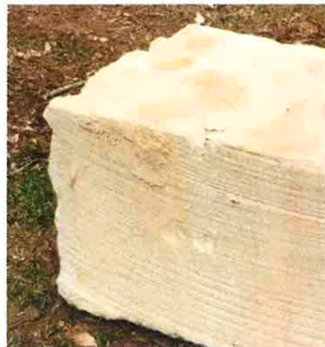
Sawn sandstone blocks
