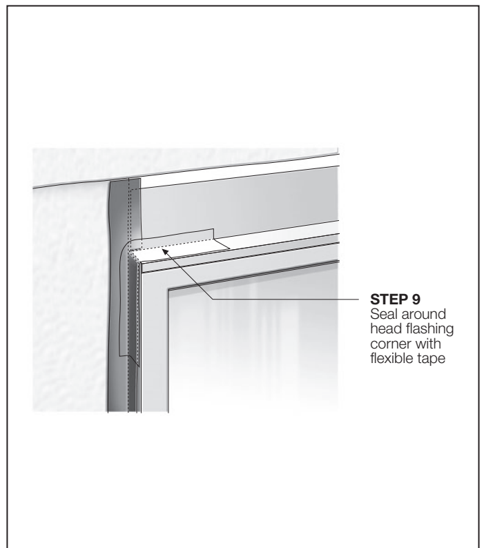
FIGURE 38 INSTALLATION OF WINDOW
