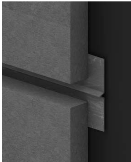
2) Closed joints where a horizontal joint profile is used to block the direct line through the joint.
