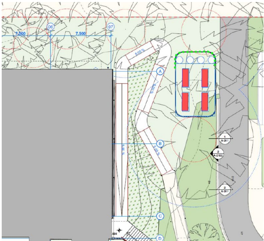
Figure 11 Location of proposed acoustic screen around mechanical plant (as shown dotted in green)
