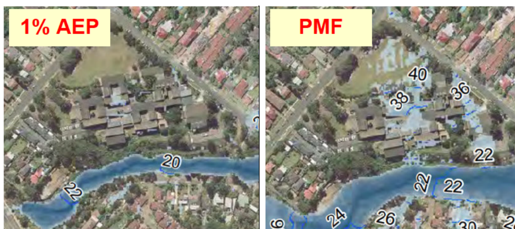
Figure 9 City of Ryde Buffalo Creek catchment flood extent study 1% AEP and PMF
