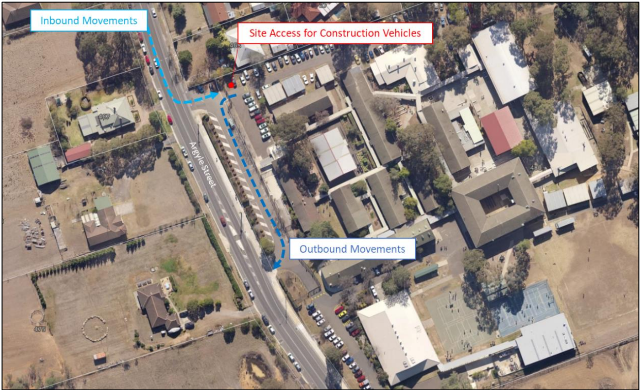
Figure 3-1: Construction Vehicle Movement Plan 1
