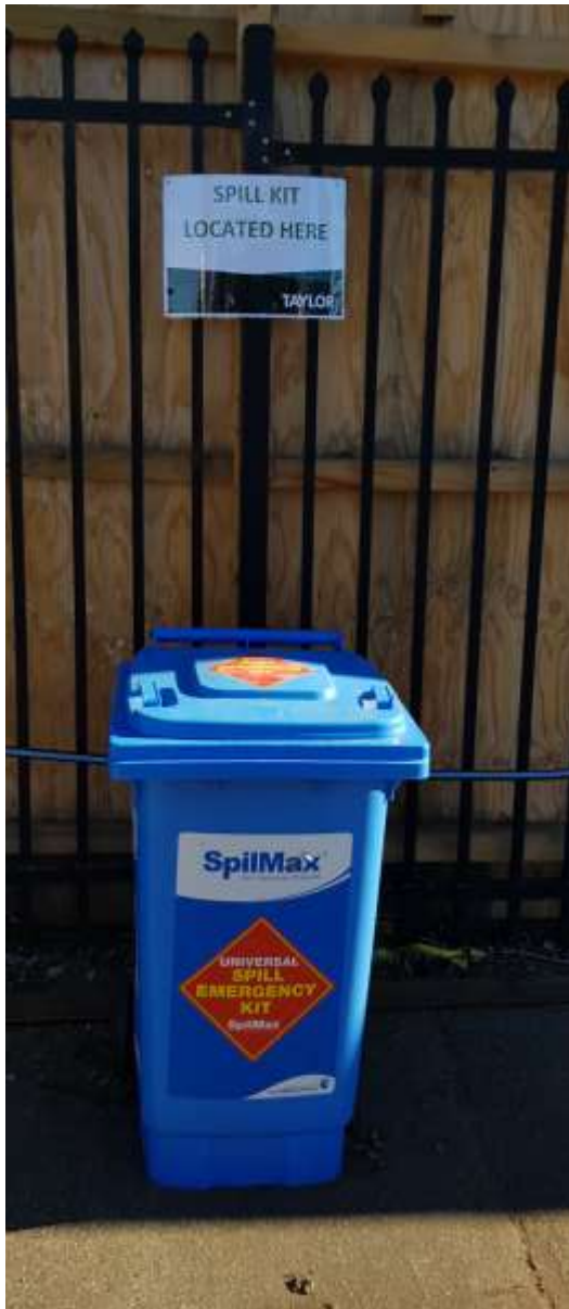
Photo 2: Spill kits, stocked and readily available
