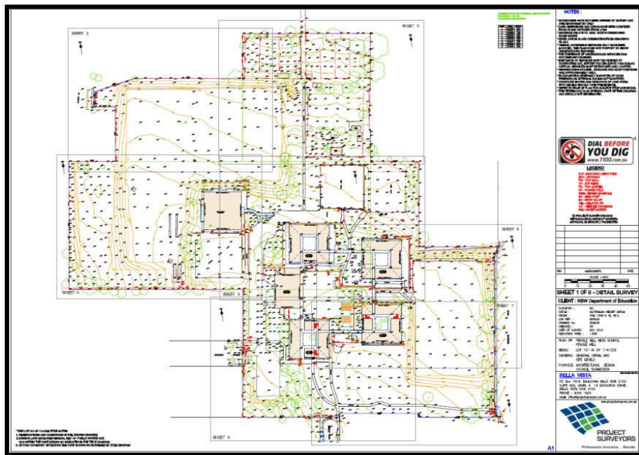
Figure 20: Site survey and contour drawing illustrating the extent of surface modification from the original surface profile.
