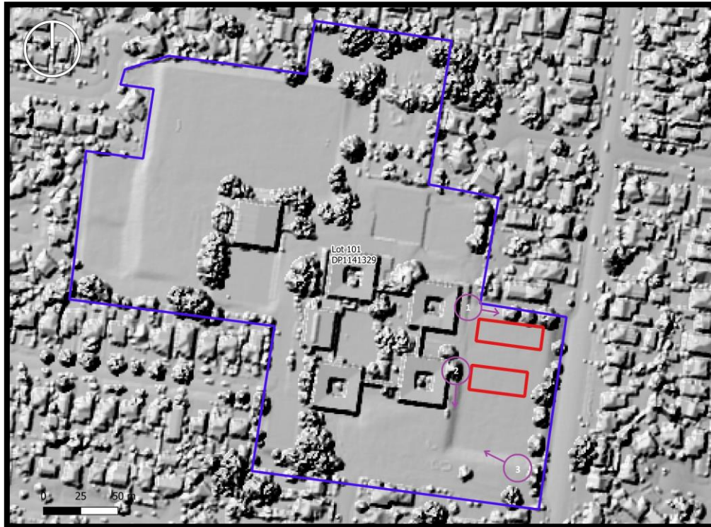
Figure 24: Hillshade image showing the position of the new buildings (red rectangles). The building are positioned on an area that has been levelled for the playing field at the school. The three following image locations and view direction are represented by circled items 1 to 3. LiDAR Sourced from the NSW Department of Customer Service, Spatial Services 2019.
