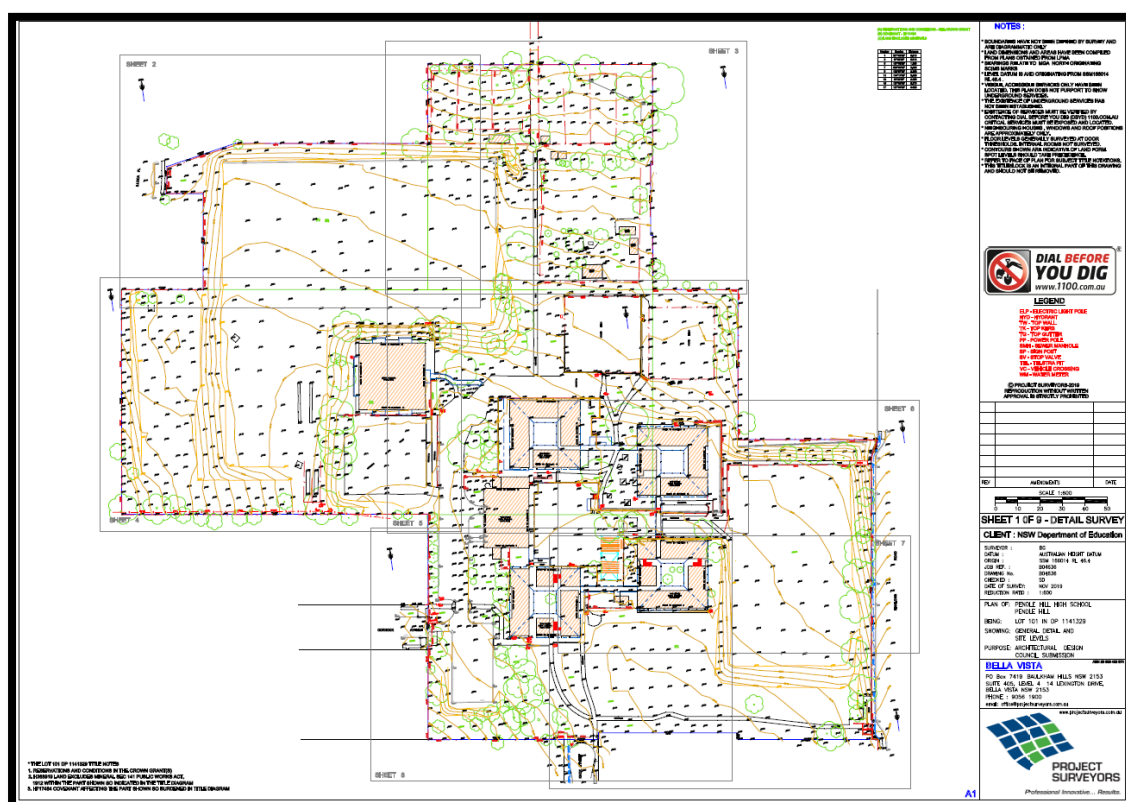
Figure 22: Site survey and contour drawing illustrating the extent of surface modification from the original surface profile.
