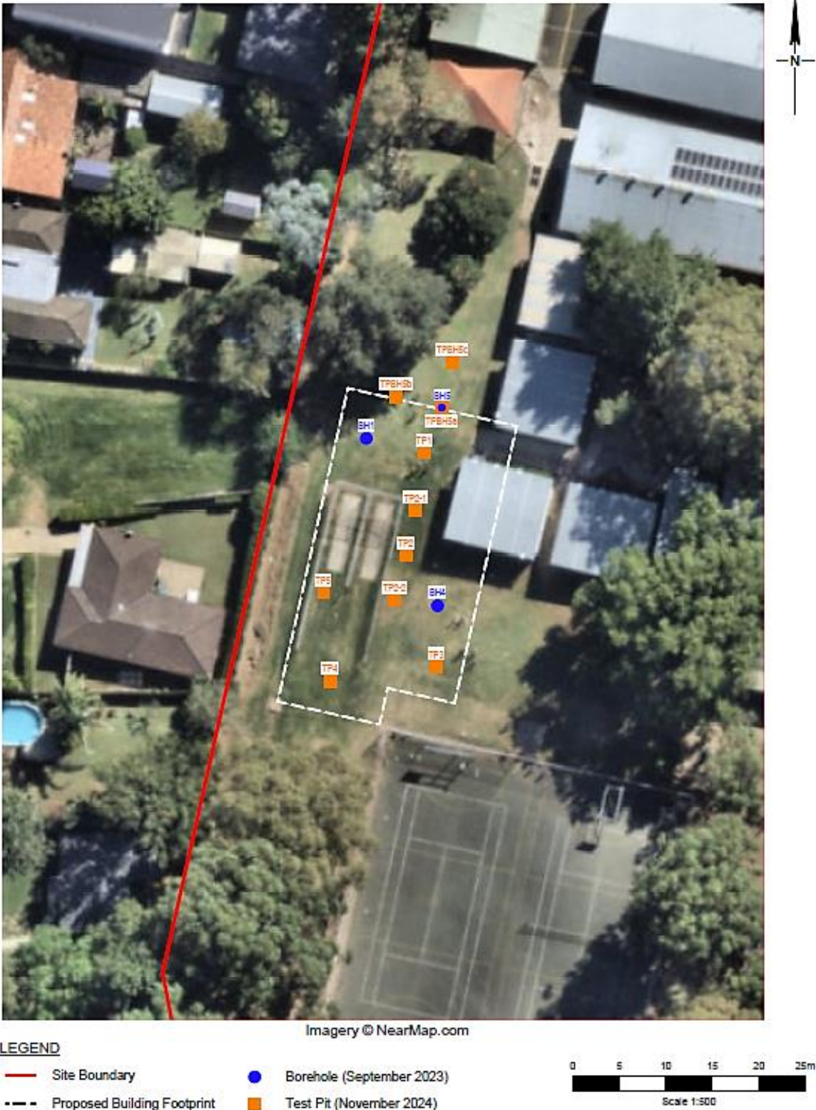
Figure 21: DSI Borehole and Test Pit Locations (Source: Geotechnique, 2024)
