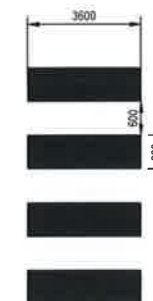
LINEMARKING FOR PEDESTRIAN CROSSING (PX)
