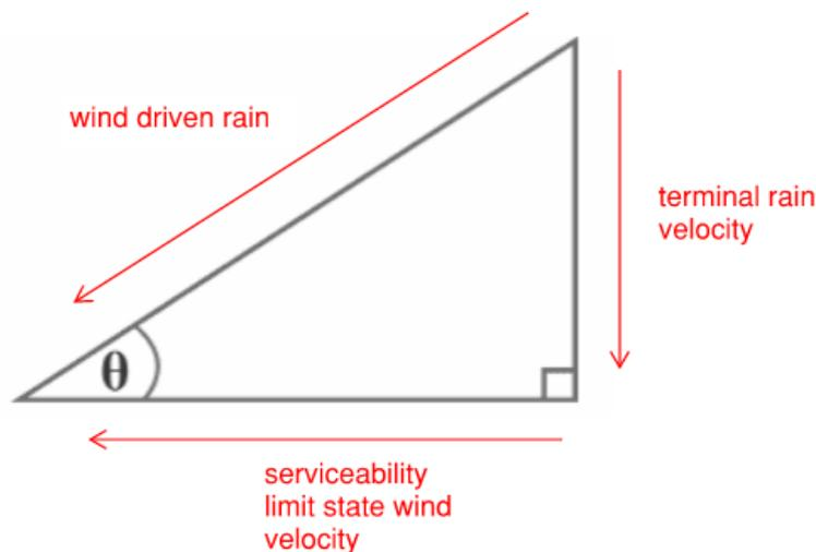
*Figure 3.5.1: Rain inclination angle illustration*
