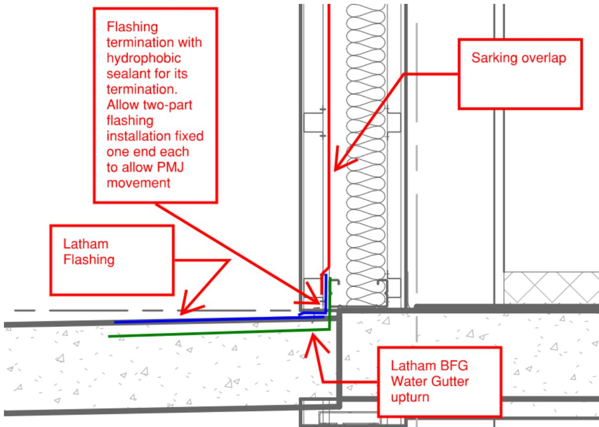
Figure 13: Section view of PMJ interface to the facade
