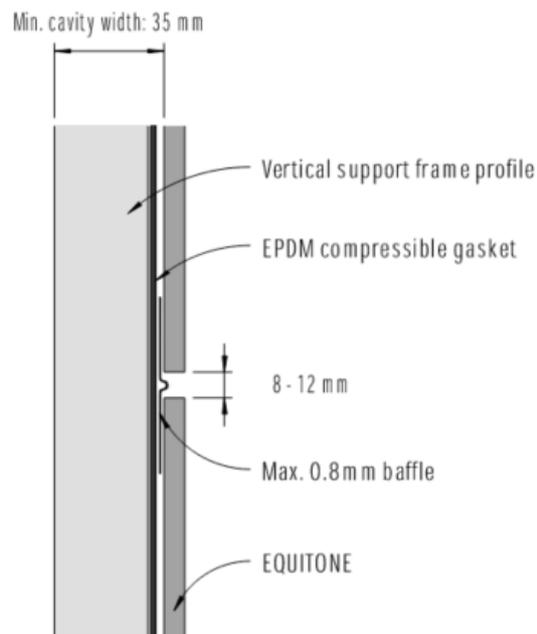
Figure 3.2: Equitone Typical Horizontal Detail
