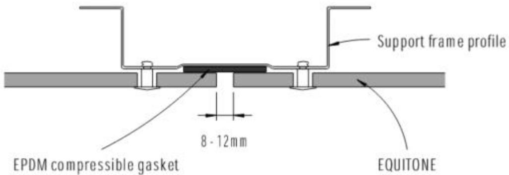
Figure 3.1: Equitone Typical Vertical Section Detail
