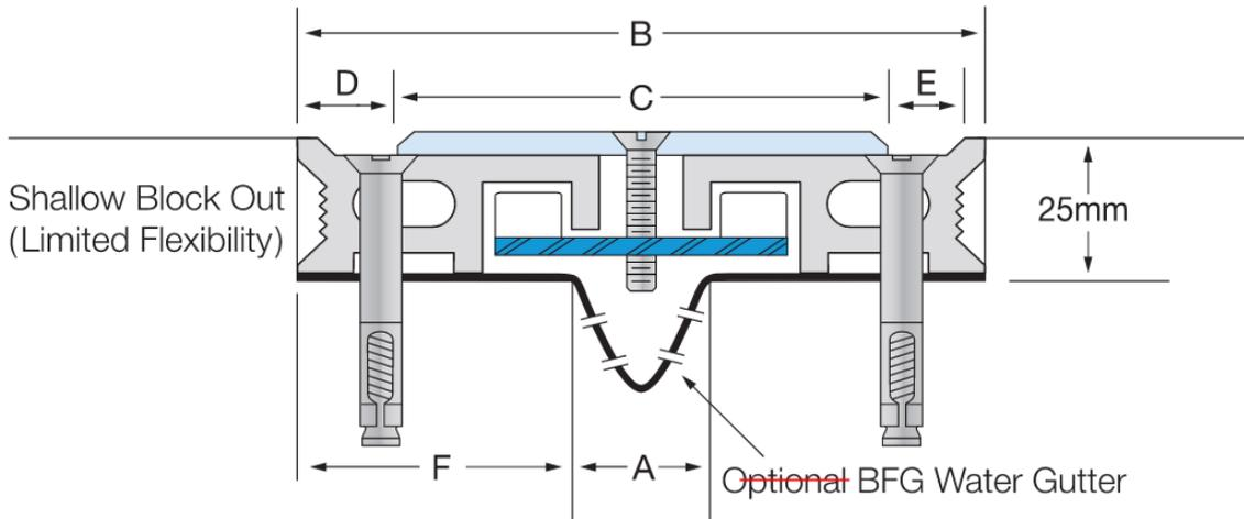
Figure 12: Latham HHS Heavy Duty Series Product, BFG Water Gutter is required.
