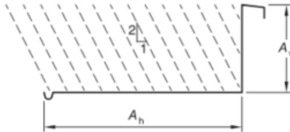
*Figure 10: Representation of the assumed rain catchment for vertical wall with flat roof/balcony in NZS/AS3500.3:2021 Figure 3.5.2(b)*
