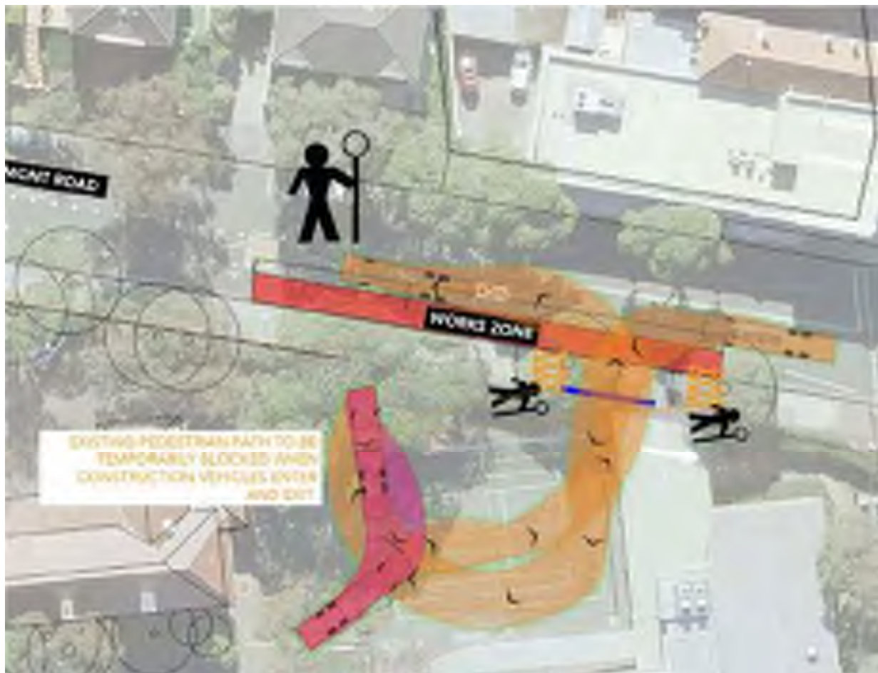
Figure 22 – Demolition Gate Access during Phase 1
