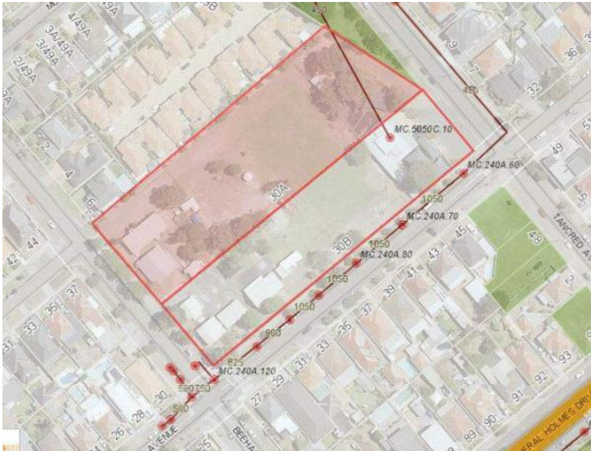
Figure 2.3.1 – Indicative External Stormwater system (Source: Bayside Council)
