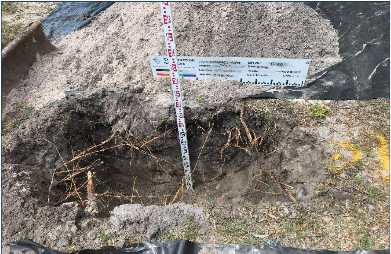
Photograph 6: TP10 location showing shallow topsoil profile over sands adjacent Jacobson Avenue.
