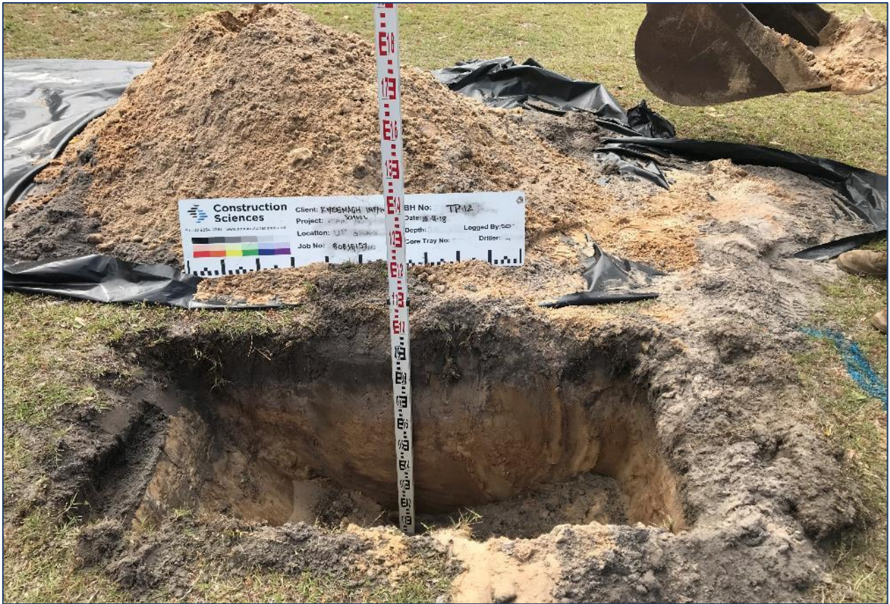
Photograph 5: TP12 location showing shallow fill and topsoil profile over sands within the open grassed area.
