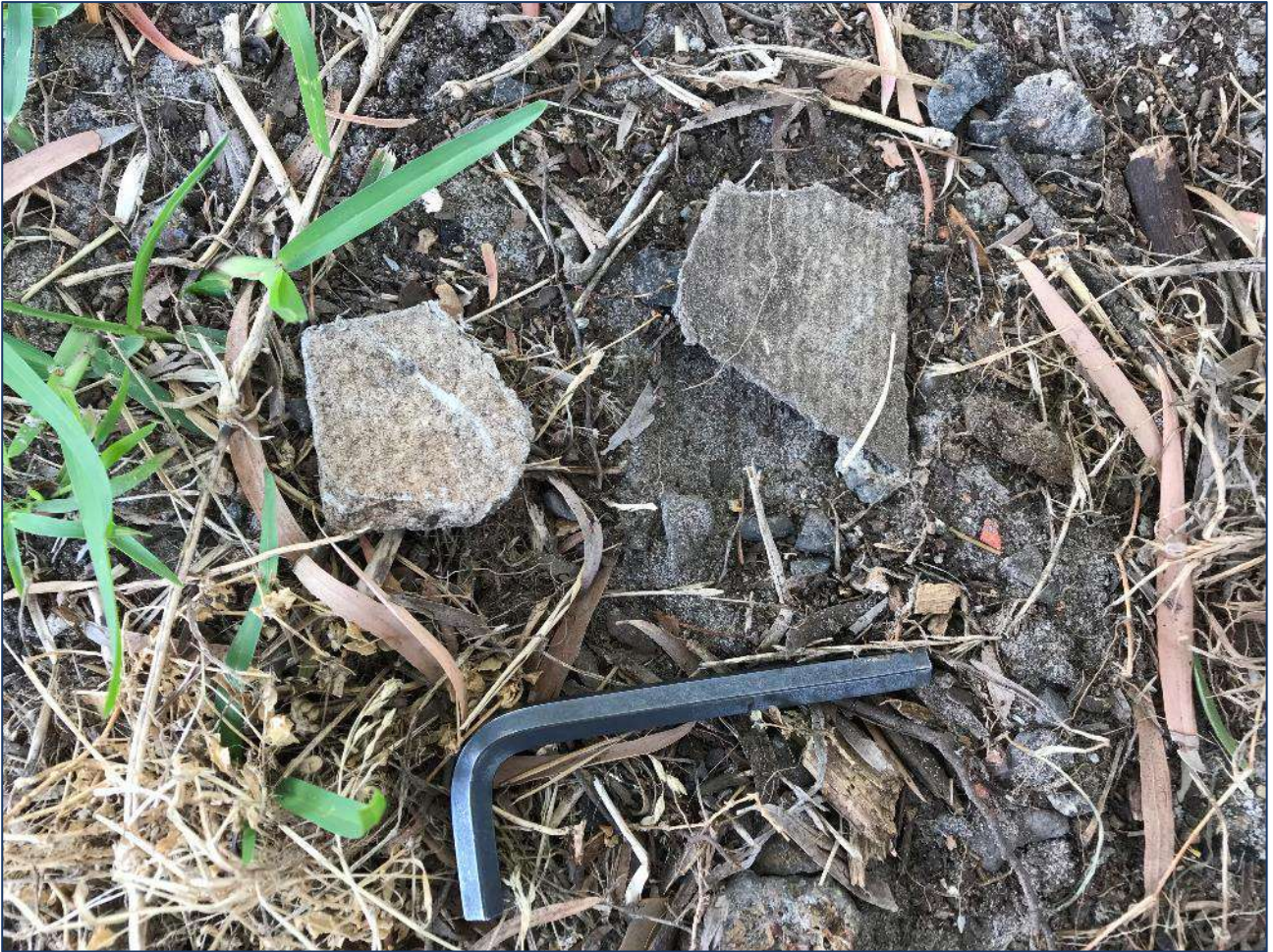
Photograph 7: ABS2 location adjacent TP19 showing representative fibre cement fragments containing chrysotile asbestos at the soil surface.
