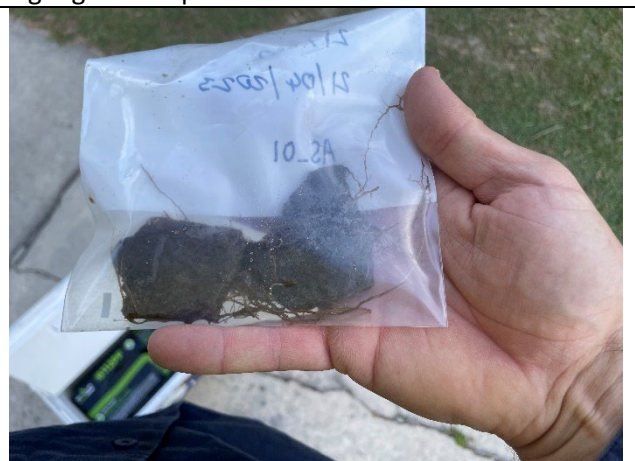
Photo 6: Asbestos fragments found within trench
