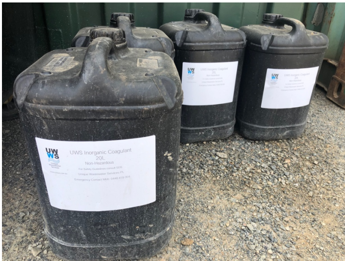
Figure 7 Flocculant drums with no clear hazard indication for handling or storage
