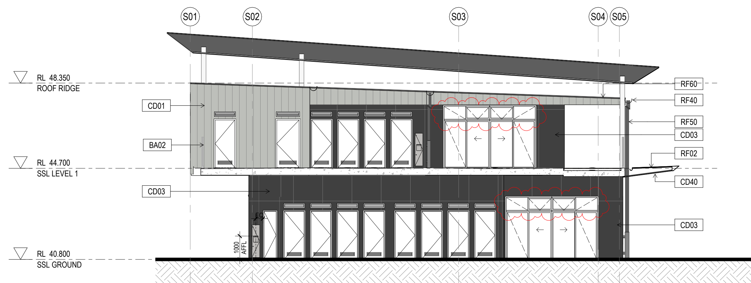
4 ELEVATION - BLOCK B3 - WEST 1 : 100
