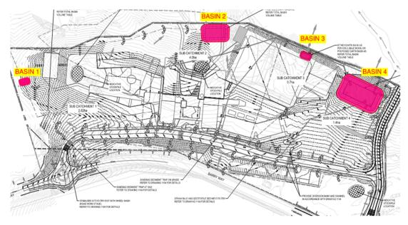
Calculations to determine the concept design basin size have been based on available geotechnical information regarding soil types and through the use of the Soils and Construction Volume 1 Manual.
