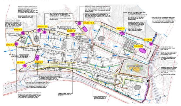
Calculations to determine the concept design basin size have been based on available geotechnical information regarding soil types and through the use of the Soils and Construction Volume 1 Manual.
