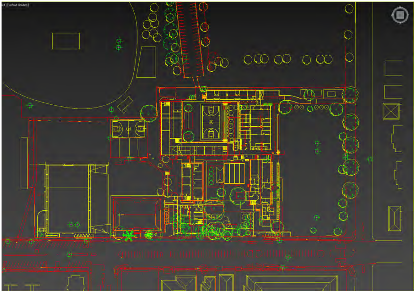
Image showing proposed survey drawing(in red lines) aligned to architectural drawing(in yellow lines)
