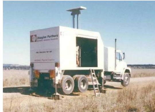
Figure 2: Purpose built CPT rig
