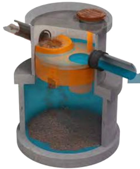
Figure 1 – HumeCeptor® system operation during design flow conditions
