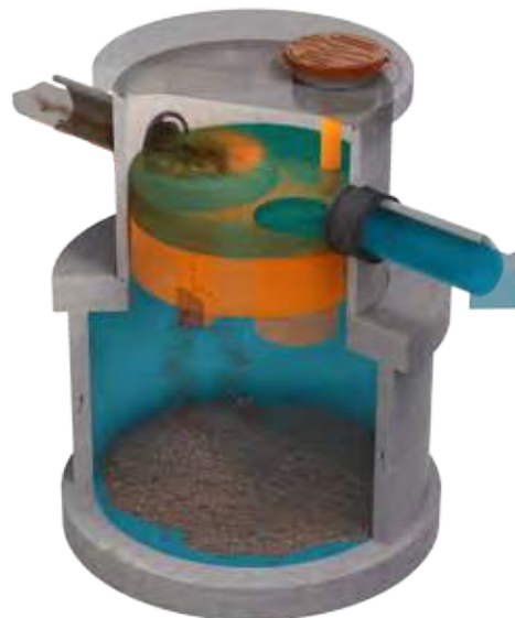
Figure 2 – HumeCeptor® system operation during high flow conditions
