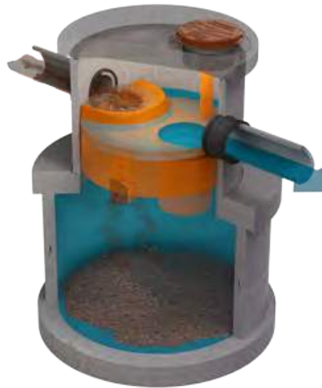
Figure 1 – HumeCeptor® system operation during design flow conditions
