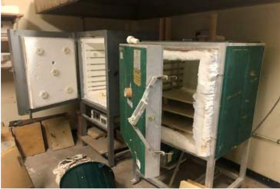
Photograph 15: B00B, BR1017, green and grey kilns, insulation, no asbestos detected by analysis, SMF detected.
