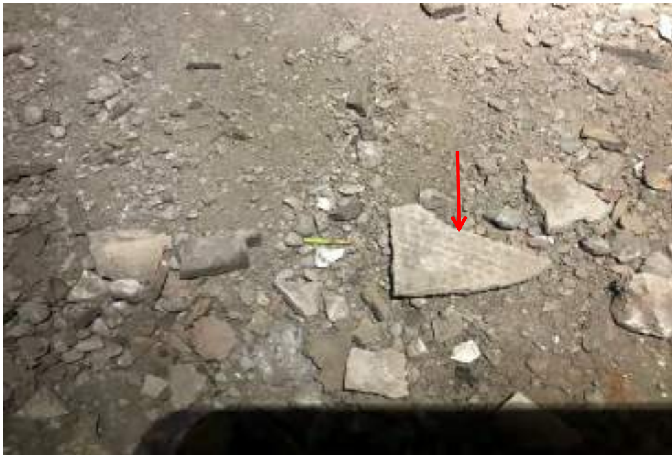
Photograph 20: B00B, subfloor, ground surface, fibre cement fragment(s), asbestos detected by analysis.
