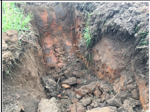
Photo 10. TP3 with visible soil profile transition on the right-hand side from silt to clay.
