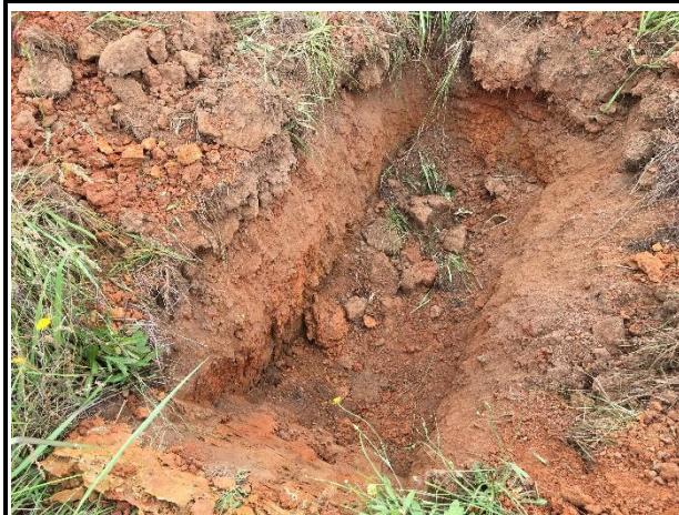
Photo 11. TP6 – minimal upper layer of silt, followed by clay characteristic of the site.
