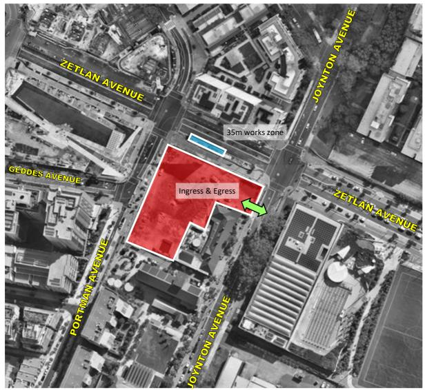
Figure 4.1: Construction site access and works zone
