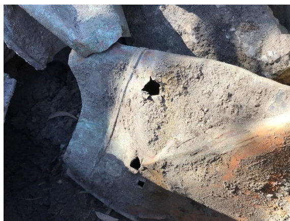
Figure 16. Detail of folded seam and two holes punched in wall of outer pan
