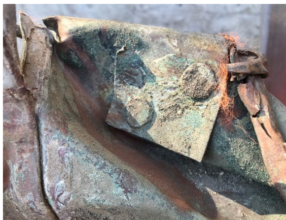
Figure 13. Hand-made rivets attaching remains of broken metal strut
