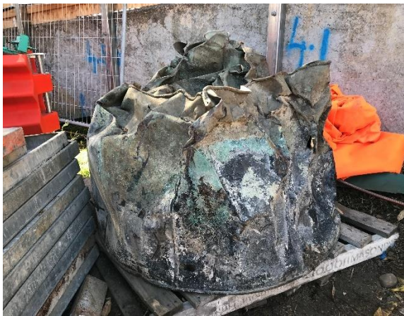
Figure 5. Side view of pans on pallet, showing folded base and side seams
