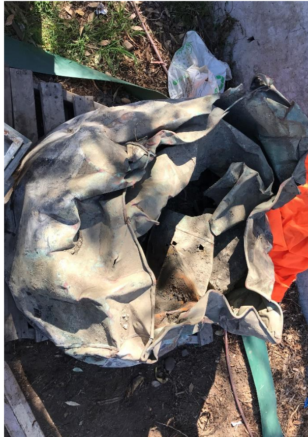
Figure 4. View of crumpled in rims of pans from above
