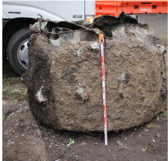
Figure 6-2 Copper basin once removed from the ground still encased in the concrete base.
