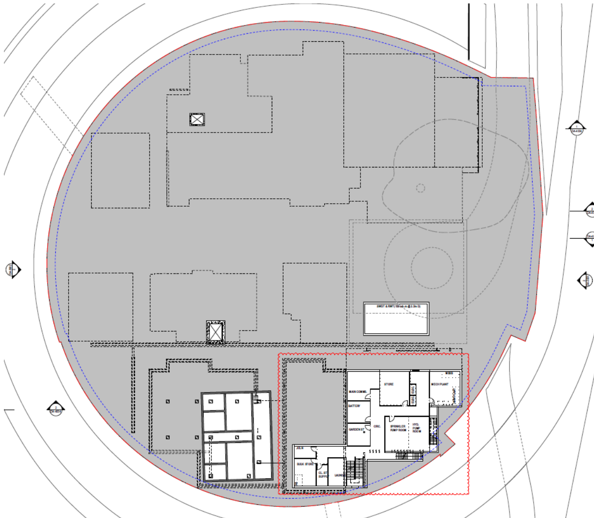
Figure 5.3: Locations of Bulk Excavation- Proposed Lower Ground Plan (Source FJMT DWG DA-2001-SSDA01, 18.10.19)
