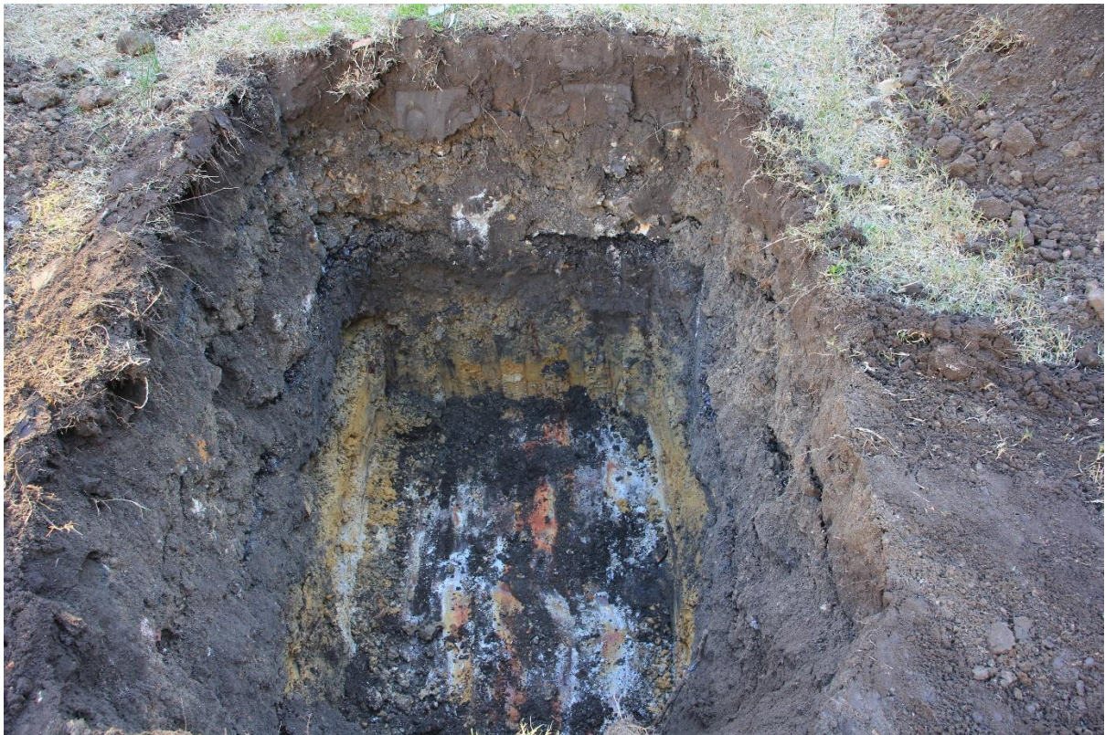
Figure 2-11. Environmental Pit 8 showing partly disturbed natural profile below bitumen surface with levelling fills above. Source: Curio, 2019.
