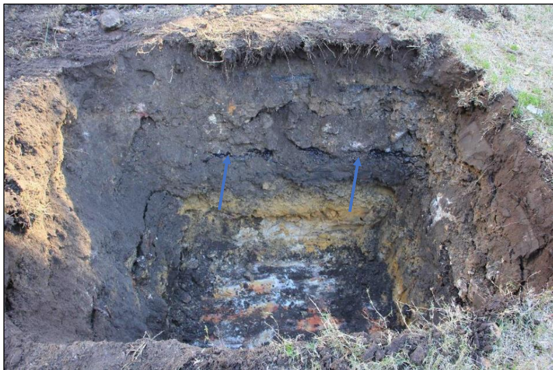
Figure 3.11: Environmental Pit 8 showing partly disturbed natural profile below bitumen surface (indicated) with levelling fills above. (Source: Curio, 2019).
