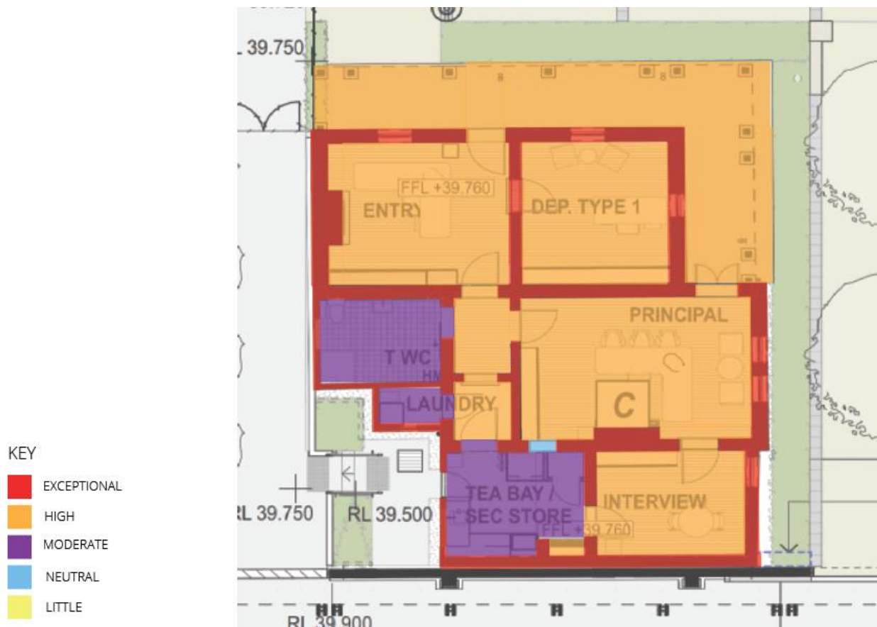
Figure 8.6: Messengers Cottage Grading of Significance plan for Internal Elements (Source: FJMT Base Plan with Curio Additions, 2023)
