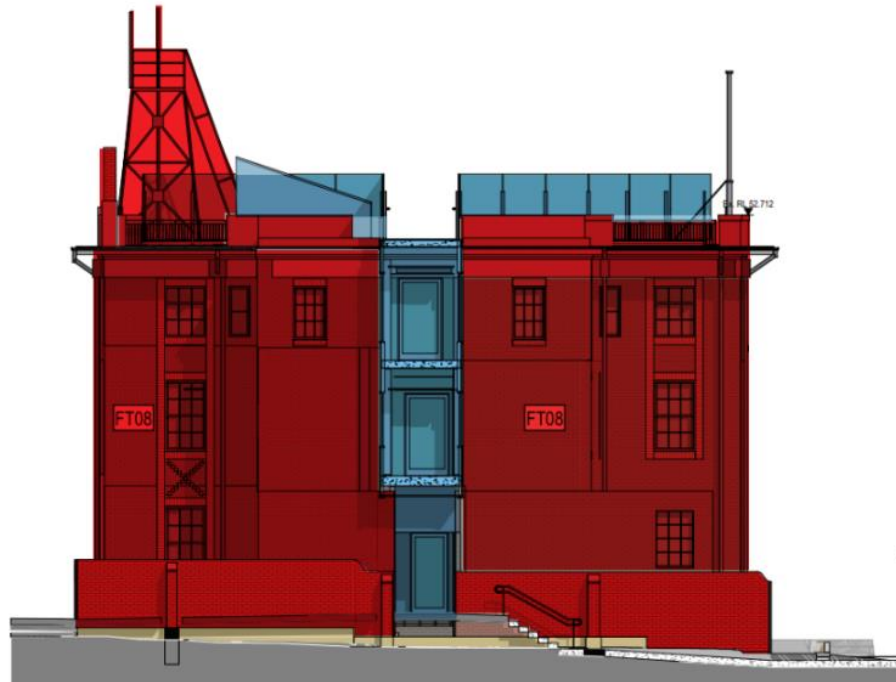
Figure 8.8: The Bureau of Meteorology Southern Façade with modern glazing highlighted in blue. (FJMT Base Plan with Curio Additions, 2023)
