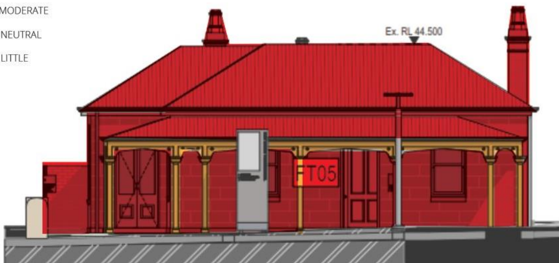
Figure 8-2: Northern Façade of the Messengers Cottage showing Gradings of Significance (Source: FJMT with Curio Projects additions)
