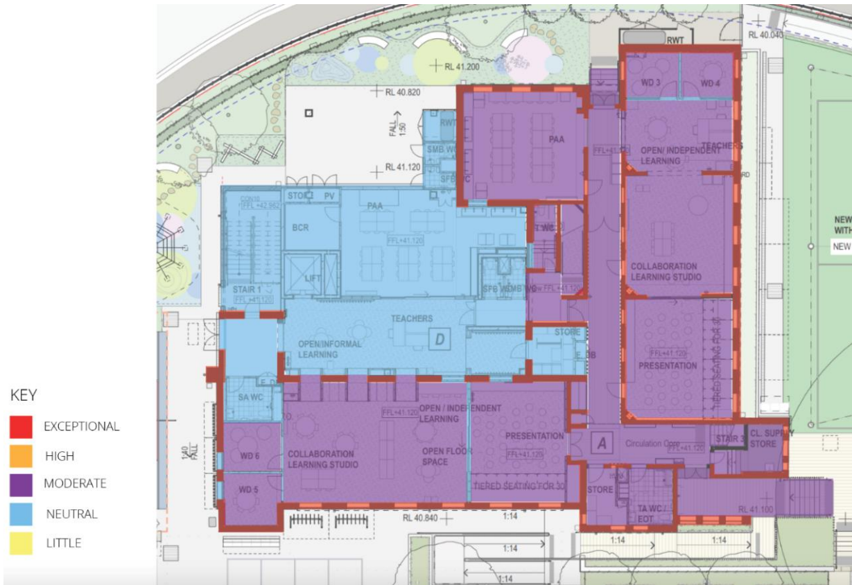
Figure 8-18: Ground Floor Fort Street Public School Ground Floor Grading Of Significance Diagram. (Source: FJMT Base Plans with Curio Additions 2023)
