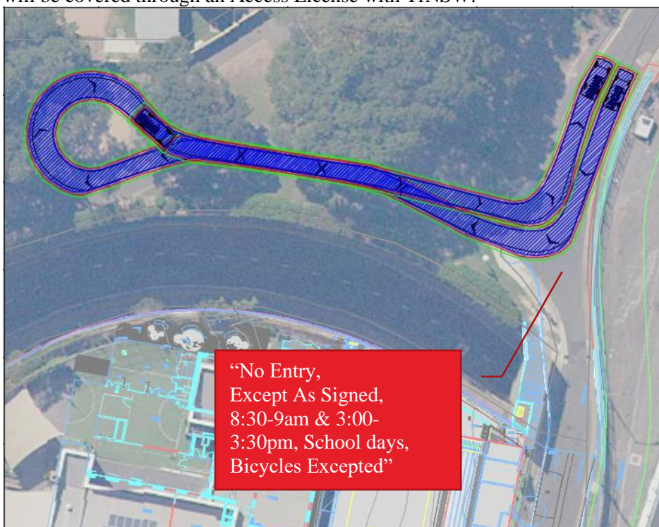
Figure 61: Southbound vehicle during gate closure turning path
