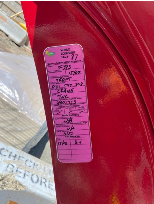
Figure 11 Lendlease plant and equipment certification sticker for 100 tonne crane
