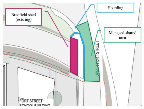
Figure 18: Bradfield Tunnel Service Shed traffic management
