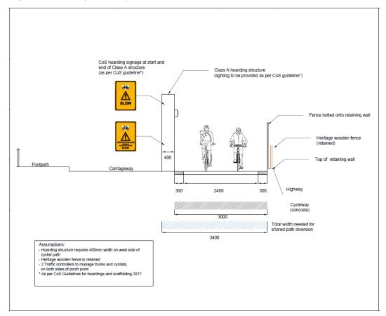
Figure 7: SHB shared path diversion hoarding structure
