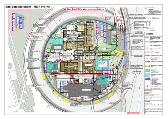
Figure 5: Hoarding and fencing boundary line for redevelopment of FSPS works
