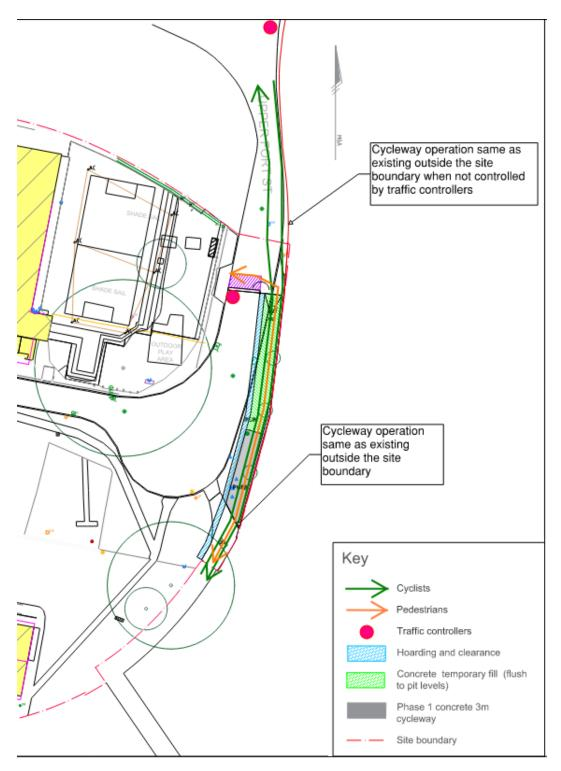
Figure 17: Operation of SHB shared path diversion
