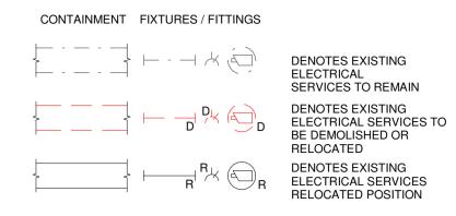
LINETYPE FOR RELOCATED OR NEW CABLETRAY/CONDUIT DETERMINED BY SYSTEM
