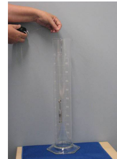
Figure 6 - lowering the sampler down the borehole (represented by the glass cylinder)
