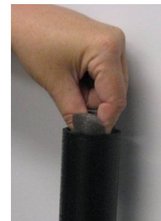
Figure 8 - insertion of compressed foam plug into the pipe
