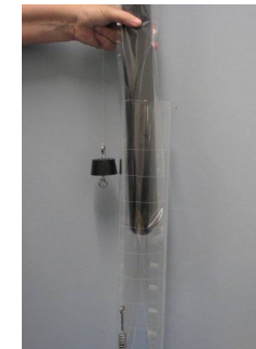
Figure 11 - insertion of pipe/foam plug and flexible plastic sleeve into borehole (represented by the glass cylinder)
