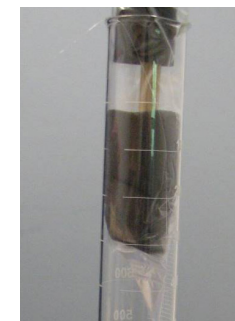
Figure 13 - extrusion of foam plug from the pipe, approximately 6 inches above the WMS-LU™ sampler
