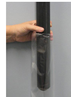
Figure 9 - insertion of the pipe, with foam plug at bottom, into plastic sleeve
