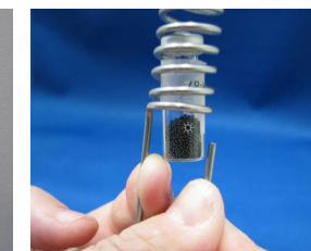
Figure 15 - removal of WMS-LU™ sampler from wire hanger
