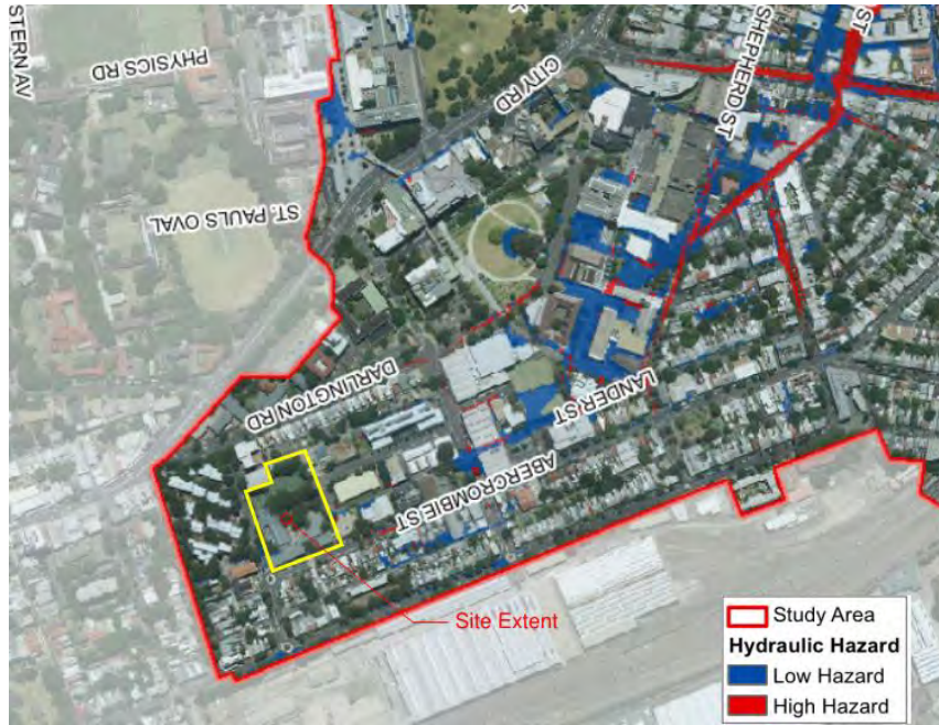
Figure 12 Flood Map – 100 Year ARI Design Flood Event (WBA Water dated September 2015)
