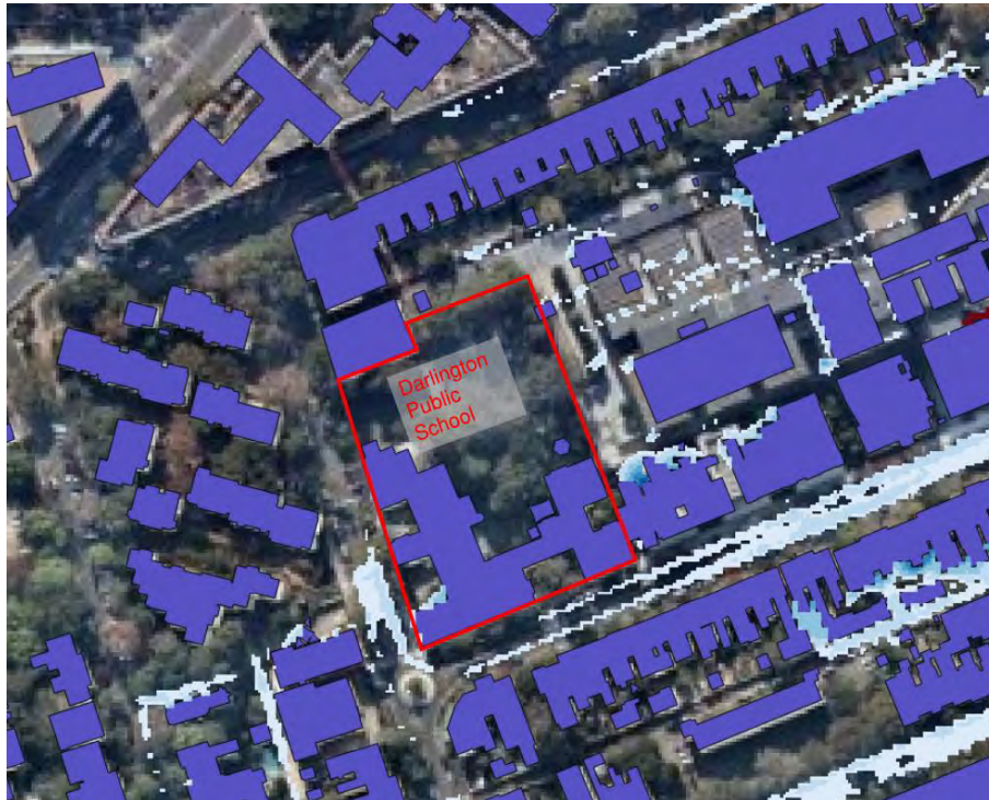
Figure 14 Flood Extent - 100 Year ARI (with 50mm Water Depth Cut-off)
