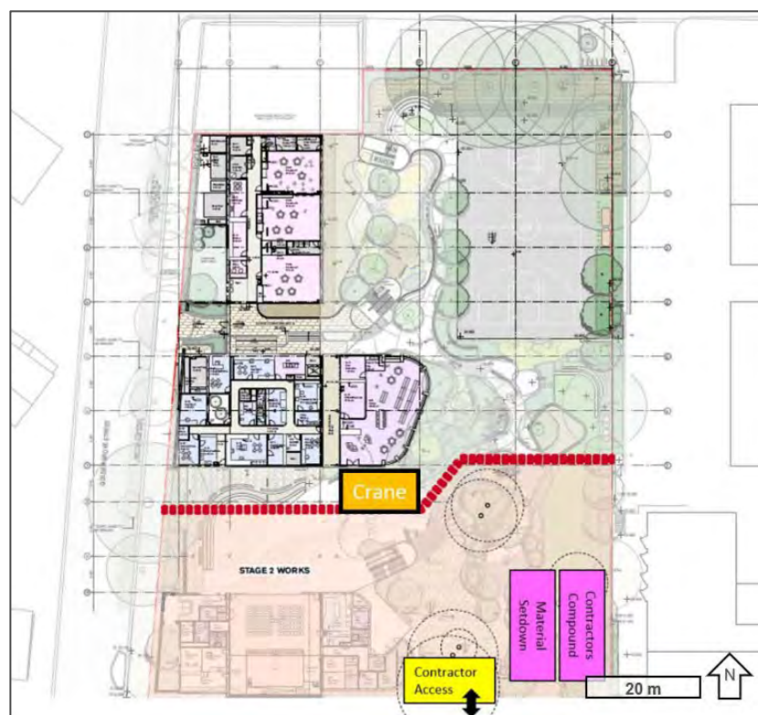
Figure 14 | Stage 2 Construction Plan (Source: Applicant's EIS 2020)
