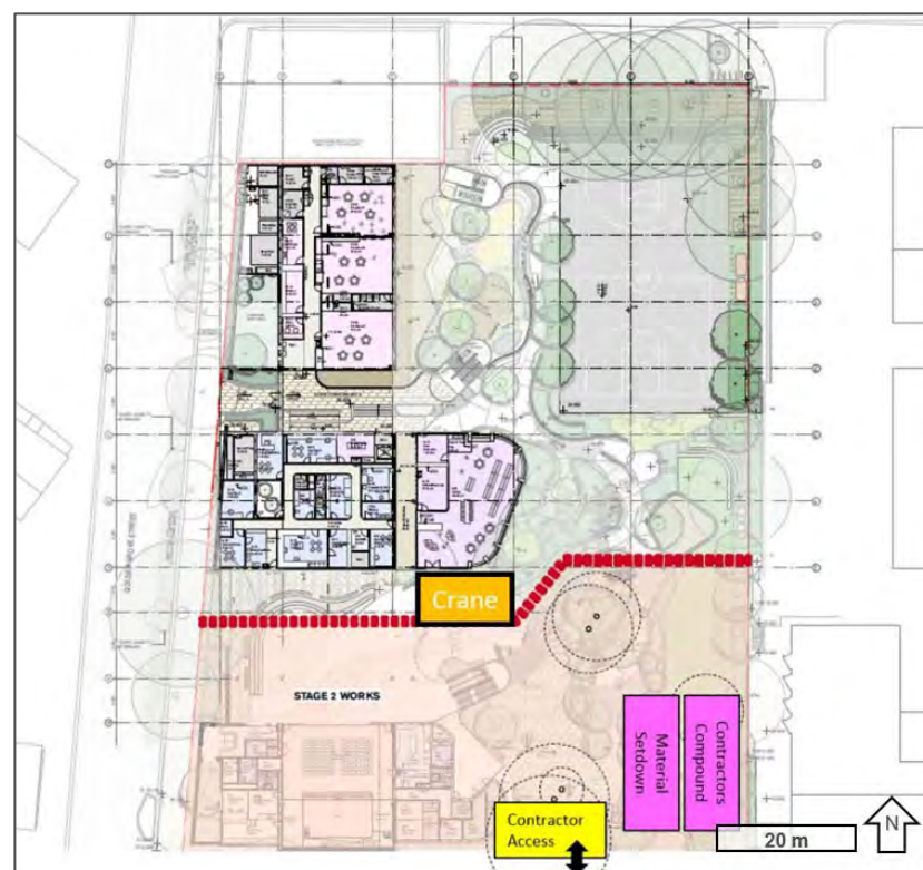
Figure 14 | Stage 2 Construction Plan (Source: Applicant's EIS 2020)
