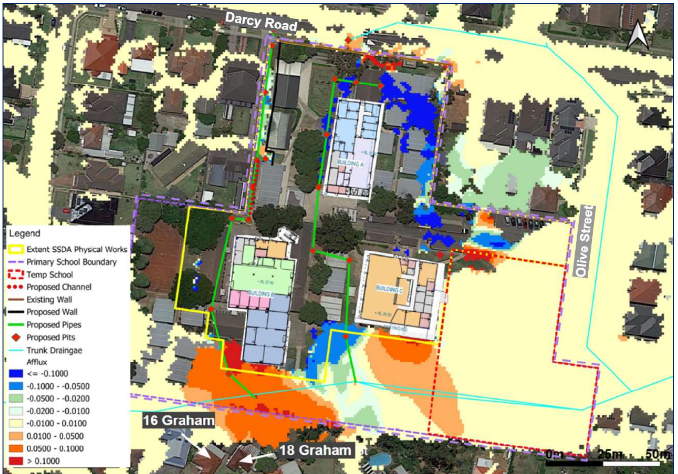
Figure 26 | Post development afflux –PMF event (Base source: Applicant’s RtS 2023)
