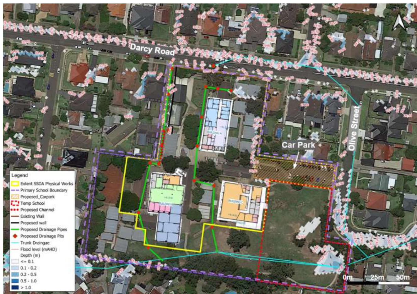
Figure 29 | 5% AEP post development flood depth and level (Source: Applicant's RtS 2023)
