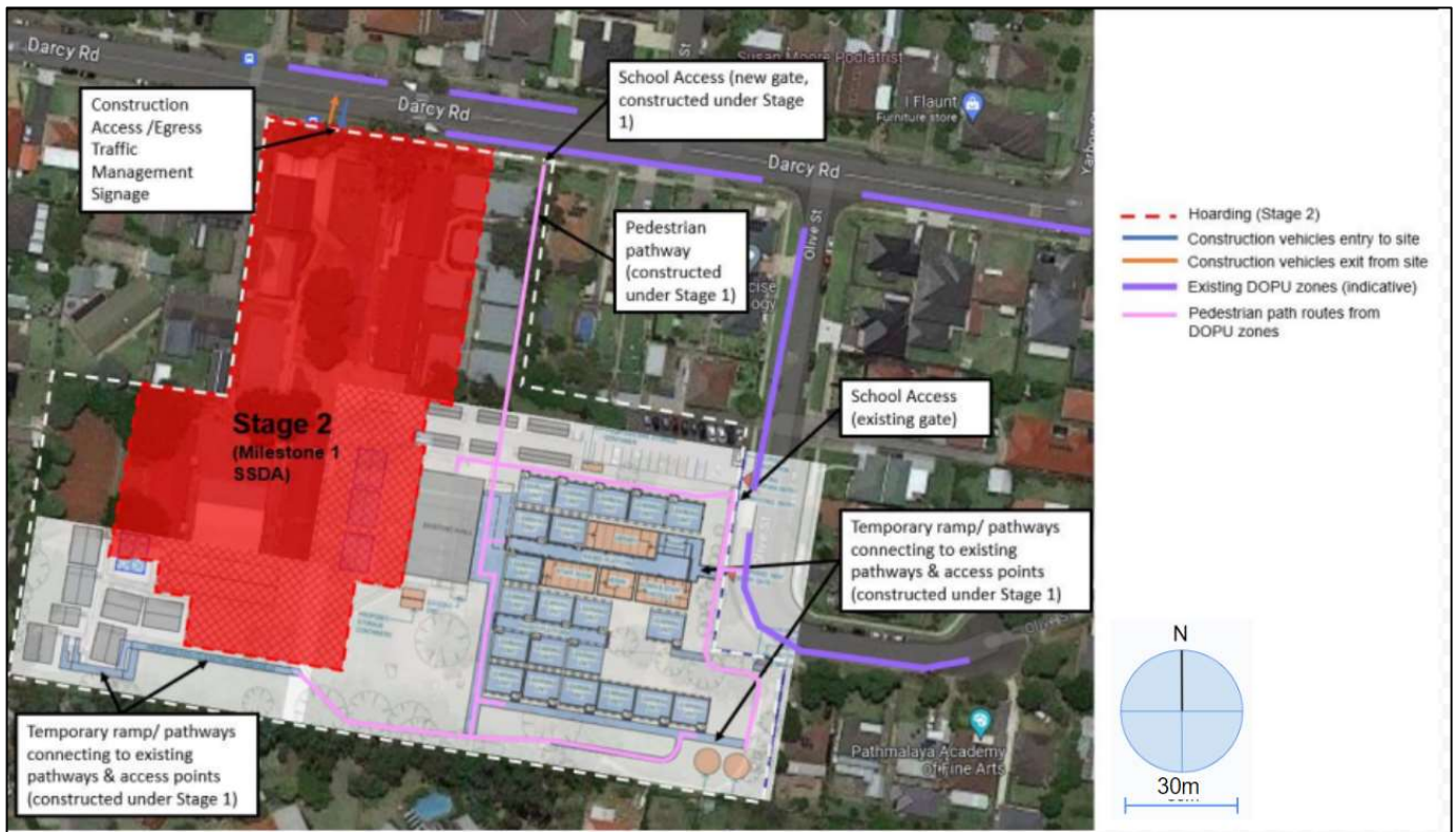
Figure 13 | Stage 2 site arrangements (Base source: Applicant's RtS 2023)
