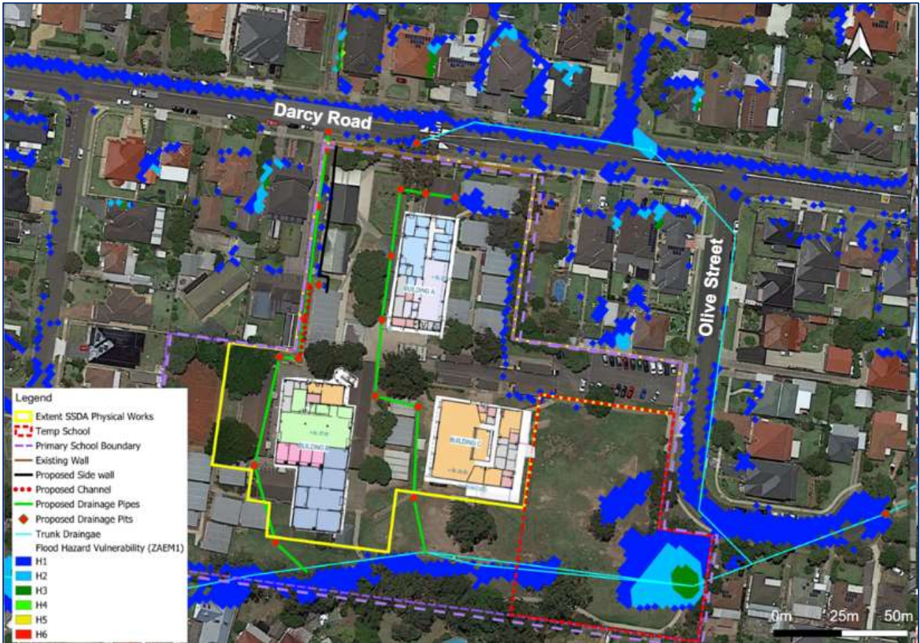
Figure 22 | Post development 1% AEP flood hazard (Source: Applicant’s RtS 2023)
