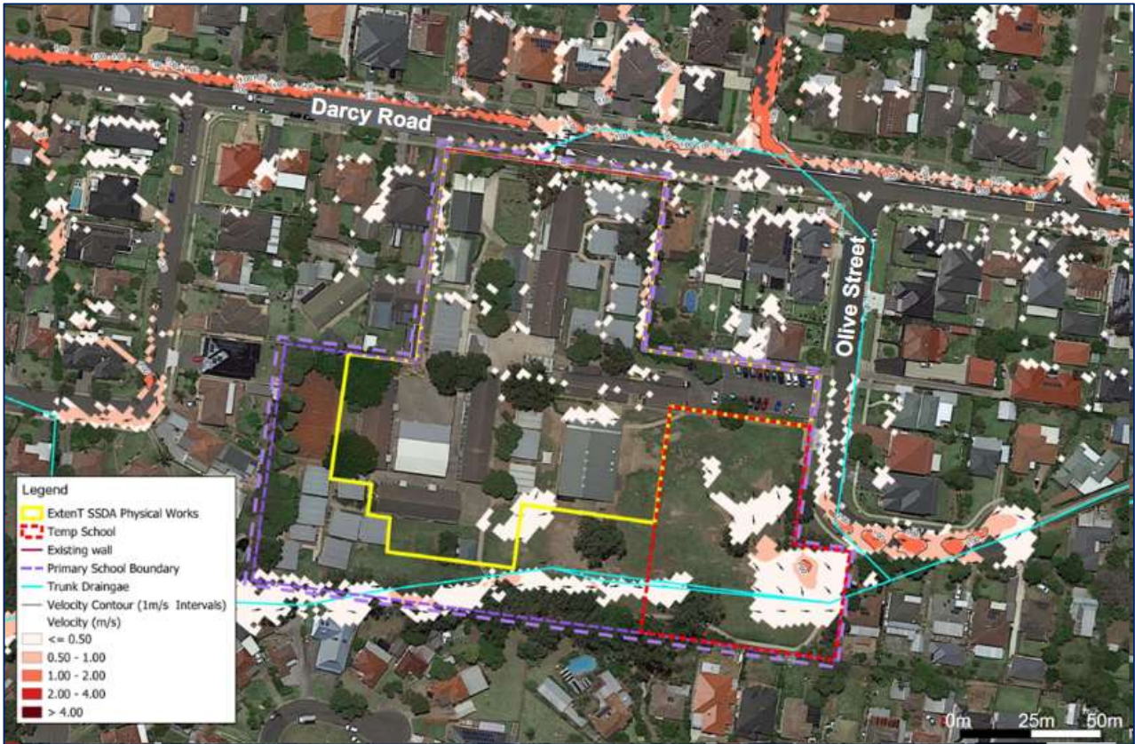
Figure 17 | Existing 1% AEP flow velocity (Source: Applicant's SRtS 2024)
