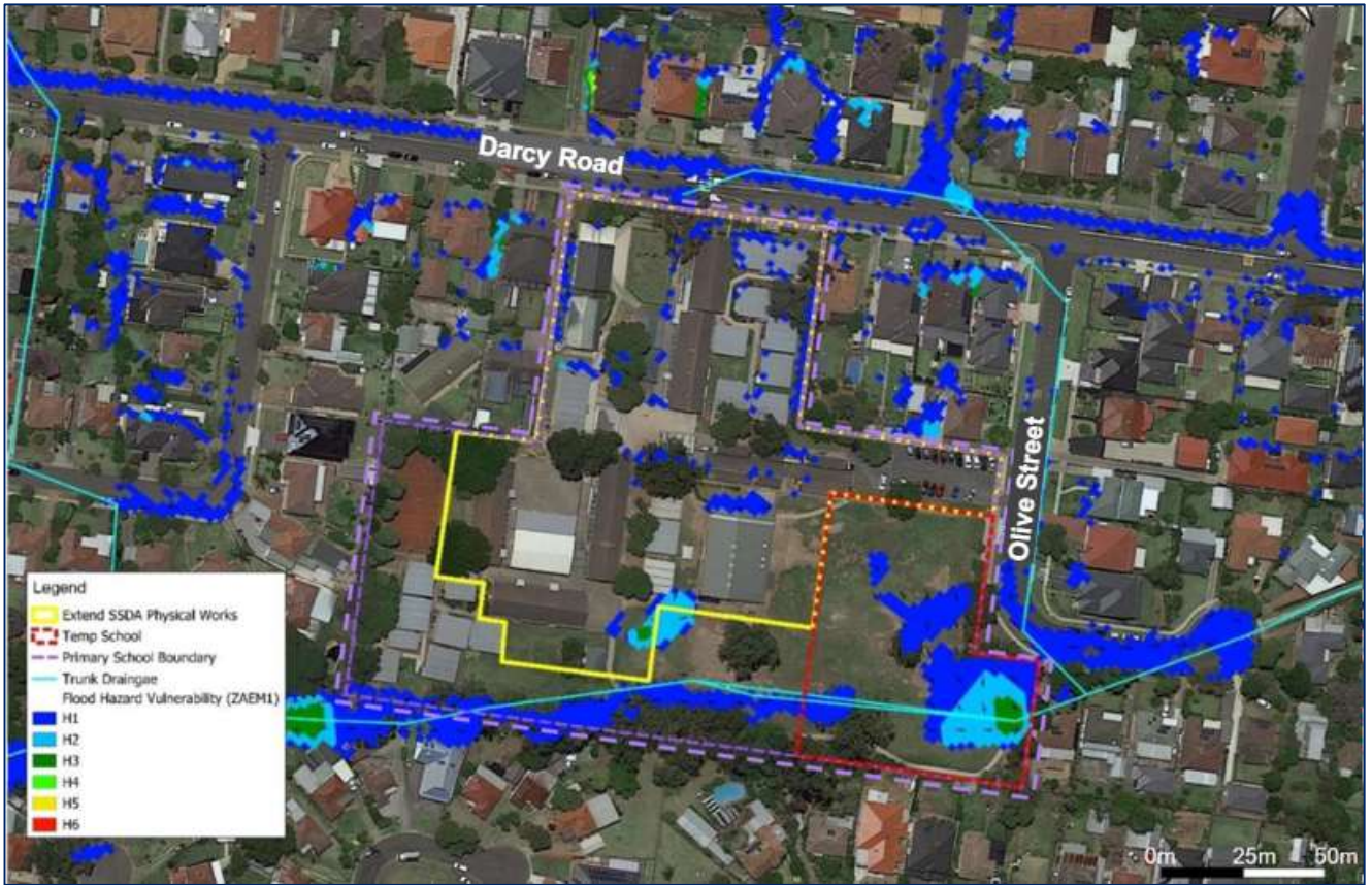
Figure 21 | Existing 1% AEP flood hazard (Source: Applicant's SRtS 2024)
