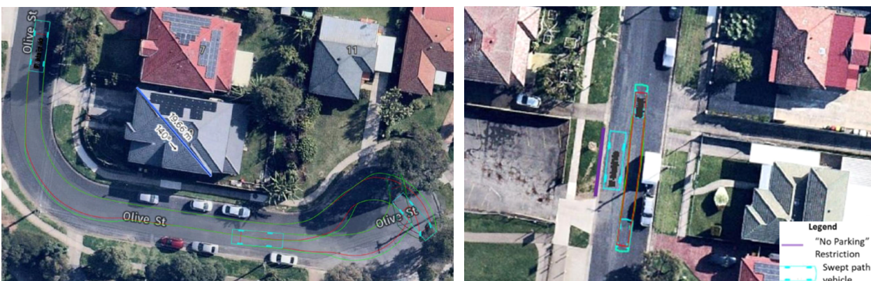
Figure 11 – Proposed Waste Vehicle Manoeuvrability for Waste Collection during Stage 3 and future state
