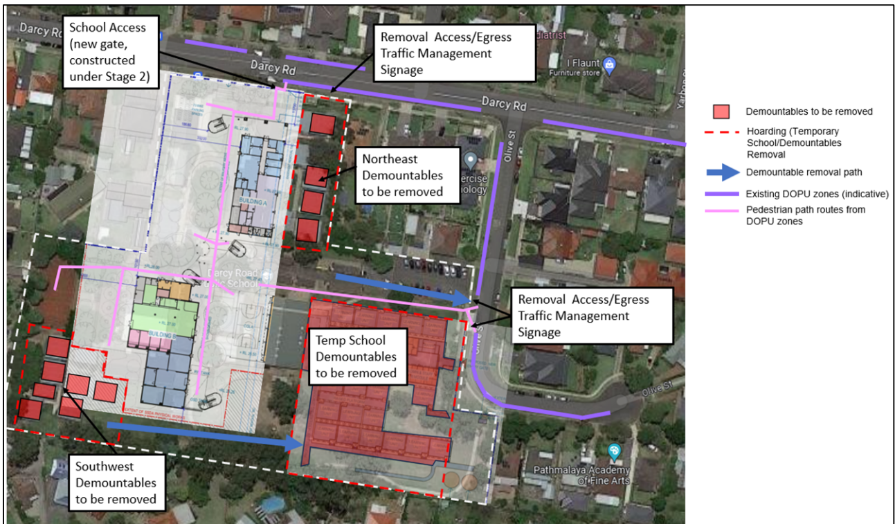
Figure 8 – Site plan during temporary school/demountable removal period (routes TBC following crane lift study)
